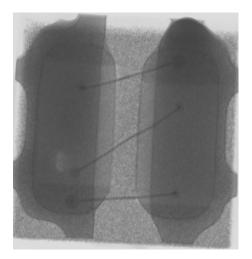
77. As reflected by x-ray images of the "flat no lead" packaged LED device in the Journi product, in accordance with claim 1 of the Jaeger '282 patent, the entire connection carrier
