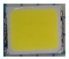
61. At least part of the thixotropic agents in the Awake and Alert BR-30 LED device are in the form of nanoparticles having a d<sub>50</sub> value, measured in Q3, that is greater than or equal to 5nm and less than or equal to 15nm, as required by claim 1 of the Braune '956 patent. Such thixotropic agents are evidenced by the lack of sedimentation in the phosphor. An example of
