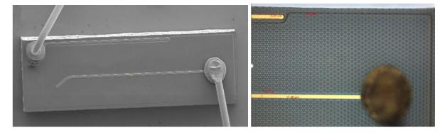
111. As further reflected by additional Scanning Electron Microscope images at a FIB (Focused Ion Beam) cut through the p-current spreader structure below of the packaged LED device in the GoodDay product, in accordance with claim 24 of the Fehrer '519 patent, the GoodDay product has an injection barrier formed between the contact and the active region; a current spreading layer, which is electrically conductively connected to the contact and which is
