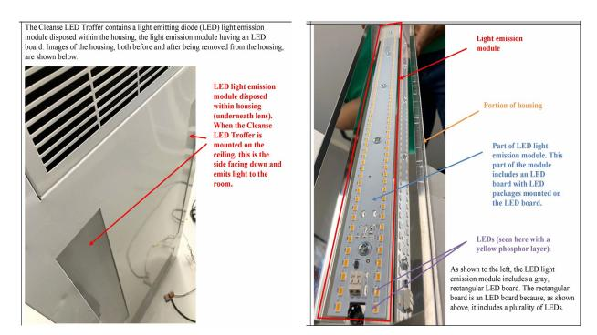
The light emission module of the Cleanse LED Troffer contains a monolithic substrate having a first side and a second side. The substrate is monolithic because it is one continuous piece of material.
