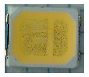
41. A scanning electron microscope image of an exemplary packaged LED device sized 2835 and having a sedimented phosphor found in the GoodDay A-19 product is provided below:
