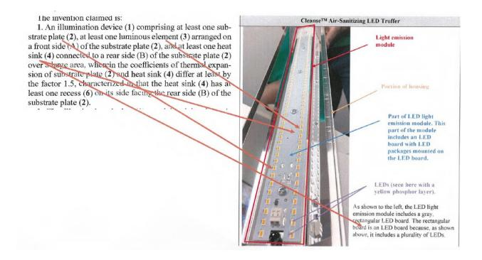
84. As reflected by Defendants' representations from the ITC complaint, the illumination device included within the Cleanse Troffer product, in accordance with claim 1 of the Kraus '146 patent, in the illumination device the coefficients of thermal expansion of substrate plate (2) and heat sink (4) differ at least by the factor 1.5, characterized in that the heat sink (4) has at least one recess (6) on its side facing the rear side (B) of the substrate plate (2) as
