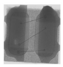
75. The "flat no lead" packaged LED device in the Journi product, in accordance with claim 1 of the Jaeger '282 patent, includes an optoelectronic semiconductor chip attached and
