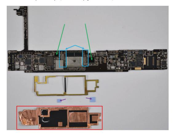
227. The '129 Infringing Products' heat spreader assembly also includes a second heat spreader interposed between the heat spreader and only one of the at least two spaced chips. For instance, the Apple iPad Pro's heat spreader assembly includes a second heat spreader (outlined in orange), which is interposed (indicated with yellow arrows) between the heat spreader and only one of the at least two spaced chips (outlined in green), as shown below:
