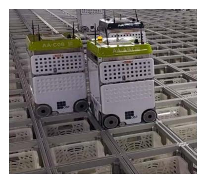
9. Because Ocado's single-space robots have greater freedom to move on top of the grid, the robots can be managed by more complex "air traffic control" software, which has a much greater probability of identifying an available traffic route that will be most efficient for item storage and retrieval (*e.g.*, relative to the constrained movement of Defendants' cantilever robots).
