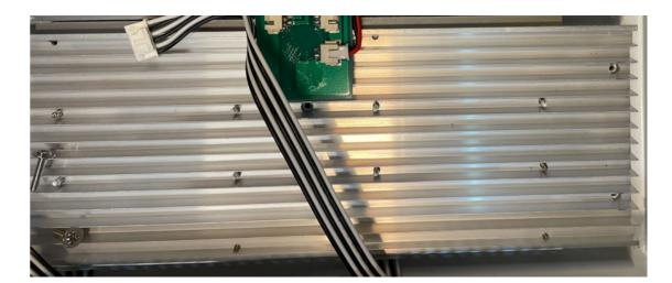
75. On information and belief, XL300 products include a housing element including fastening means for detachably coupling the housing element to the heat dissipation element; for example, XL300 products include a housing element, formed by a metal frame and secondary optical lenses. The housing element further includes threaded bores and screws to detachably couple the housing element to the heat sink.
