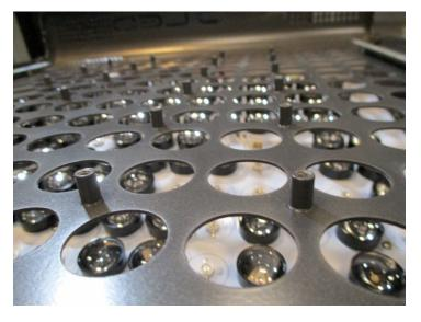
83. On information and belief, the substrate is enclosed between the heat dissipation element and said housing element; for example, the metal-core printed circuit board is enclosed between the heat sink and the metal frame and secondary optical lenses.
