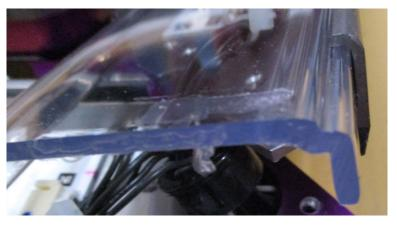
98. On information and belief, the substrate is enclosed between the heat dissipation element and said housing element; for example, the printed circuit board is enclosed between the transparent window and the heat sink.
