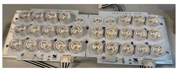
74. On information and belief, XL300 products include a heat dissipation element thermally coupled to the thermally conductive substrate; for example, XL300 products include a heat dissipation element formed by a heat sink, which is thermally coupled to the metal-core printed circuit board.
