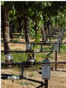
Double drip line with control electronics.
