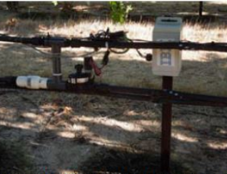
Control electronics box and node
