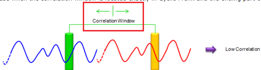
< Fig 1 : a case when the correlation window is located exactly in Cyclic Prefix and the ending part of the symbol >
