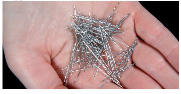
Helix's patented concrete reinforcing Micro Rebar<sup>TM</sup> results in stronger, more durable, and more flexible concrete than traditional rebar, with improved fatigue endurance, crack resistance, impact capacity, energy absorption, and shatter resistance.
