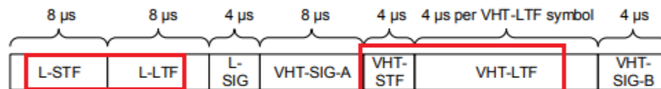
Figure 21-28—VHT NDP format
