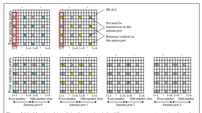
Figure 3.16 Mapping of downlink reference signals for different antenna ports (normal cyclic prefix)
