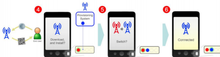
Remote SIM Provisioning Operation – Operator Profile Selection
