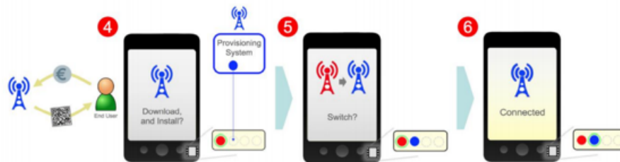
Remote SIM Provisioning Operation – Operator Profile Selection
