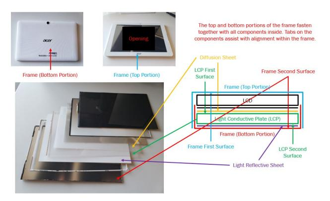
66. In the above-referenced product, the diffusion sheet and the light reflective sheet cooperate to fasten the light conductive plate within the frame, a shown below.
