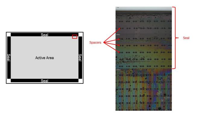
61. The Accused LCD Product has a leveling layer formed on the switching element array. As shown below, the leveling layer has an opening area and a thin region at the seal.
