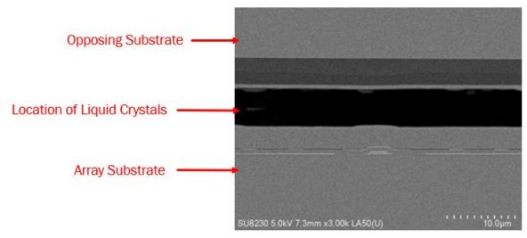
59. The Accused LCD Product has a seal across its periphery, as shown below.
