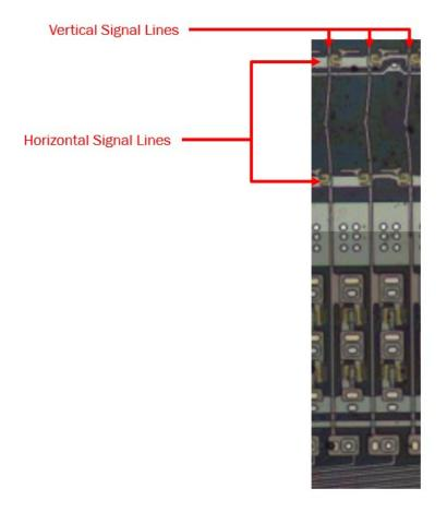
63. The surge protection circuit referenced above also includes a plurality of floating-gate field effect transistors, each having a channel capacitance and including a floating gate electrode, a source electrode, and a drain electrode. The source and drain electrodes of the transistors are connected to the vertical signal lines, as shown below.
