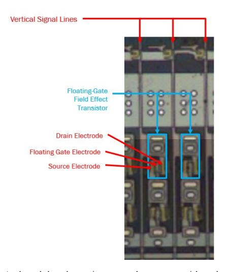
64. As shown below, the transistors respond to surge potentials on the vertical signal lines by turning on and establishing a low-impedance path to ground.
