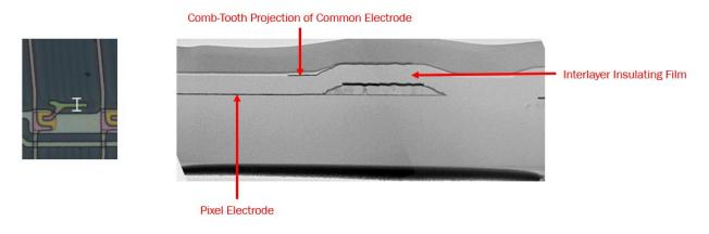
54. As shown below, in the Accused LCD Product, an alignment film and a protective insulating film are present above the pixel electrode.
