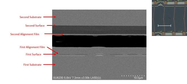
46. As shown below, the Accused LCD Product has a predetermined space is between the first and second alignment films in which the liquid crystal resides.
