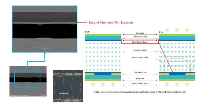
57. The Accused LCD Product has an accumulated capacitance increasing means (e.g., dielectric between the pixel electrode and comb-tooth projections of a common electrode), as shown below.
