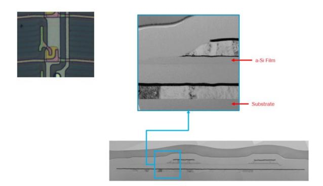
37. As shown below, aluminum source and drain electrodes are formed on the amorphous silicon with the n-type amorphous silicon film there between. The source and drain electrodes were determined to be made of aluminum (Al).
