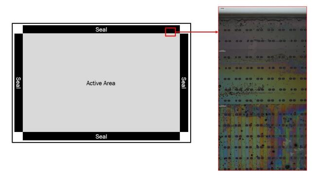
60. The Accused LCD Product has a spacer in the seal to make a gap between the array substrate and the opposing substrate constant, as shown below.
