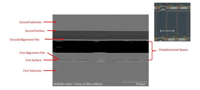
47. The Asserted Patents also cover the Accused LCD Product, because it has to have an active matrix type liquid crystal display device with two opposing insulating substrates and liquid crystal in-between, as illustrated below in reference to K&D Technology LCD Model No. KD101N37-40NA-A10, as shown below.
