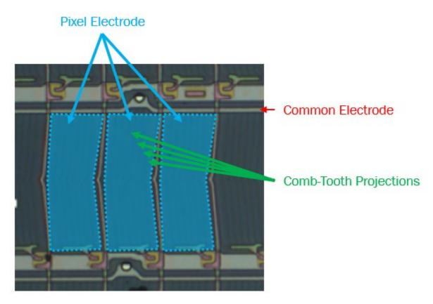
53. As shown below, in the Accused LCD Product, at least a portion of each pixel electrode is opposite to a common electrode and interposed by an interlayer insulating film. The interlayer insulating film is disposed between the common electrodes and the pixel electrodes.
