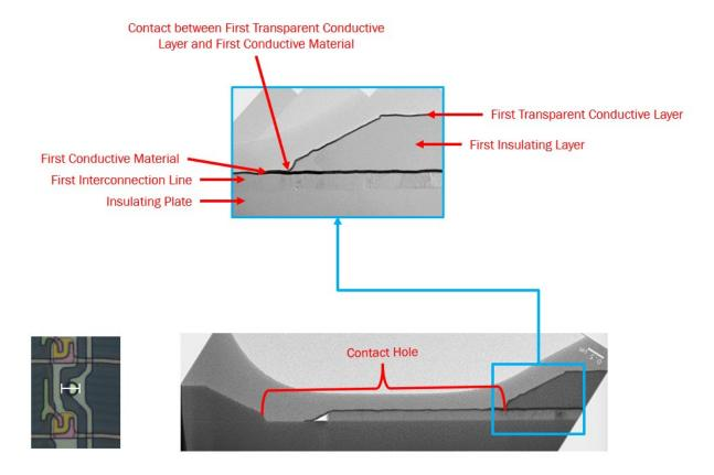
42. In the Accused LCD Product, the transparent conductive layer, first interconnection line, and first conductive material are electrically connected, as shown below.
