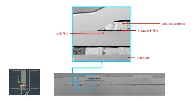
38. The Asserted Patents cover liquid-crystal display devices, as shown below, having an aluminum interconnection line disposed over an insulating plate by way of an underlying insulating layer.
