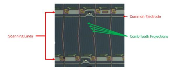
52. As shown below, the Accused LCD Product has pixel electrodes that are substantially parallel to the comb-tooth projections and located in gaps between comb-tooth projections.
