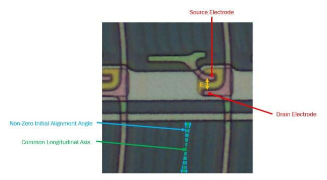
51. The Accused LCD Product also has common electrodes, as shown below, extending substantially parallel to the scanning lines and with comb-tooth projections extending toward the scanning lines.
