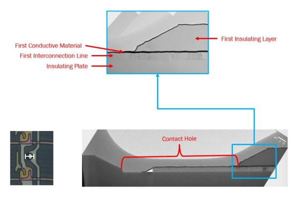
40. As shown below, a first conductive material made of ITO is in contact with the exposed part of the interconnection line and covers the whole exposed part.
