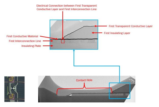
43. The Asserted Patents also cover the Accused LCD Product, such as K&D Technology LCD Model No. KD101N37-40NA-A10 (incorporated in Acer Iconia One 10 tablet), which has a first substrate with a principal surface (e.g., the inner surface), as shown below.
