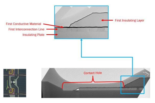
41. The Accused LCD Product has a transparent conductive layer (ITO) in contact with the first conductive material, as shown below.
