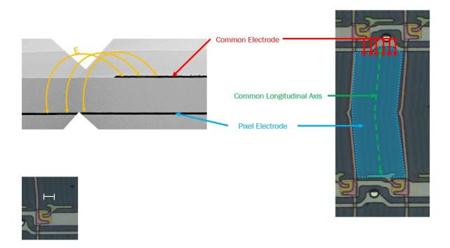
49. In the Accused LCD Product, as shown below, the liquid crystal layer has non-zero initial alignment angles relative to the common longitudinal axis and alignment of the first part of the liquid crystal layer does not change when an electric field is generated between the source and drain electrodes.
