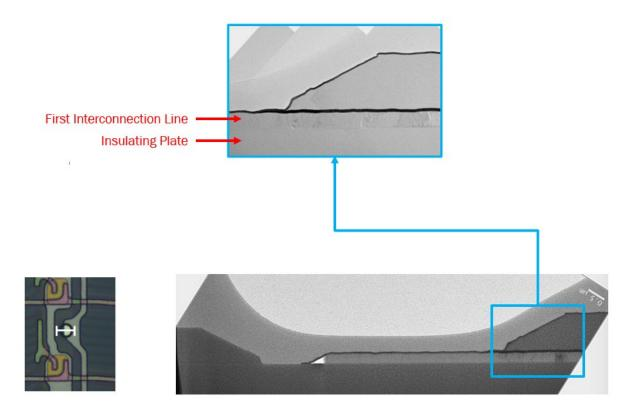
39. The Accused LCD Product, shown below, has an insulating layer that covers the interconnection line and a contact hole that exposes part of the interconnection line.
