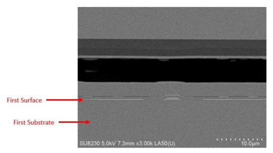
44. The Accused LCD Product, as shown below, has a first alignment film formed on the first principal surface which was subjected to an aligning treatment (necessary to set the direction of the optical/polarizing axis), as shown below.
