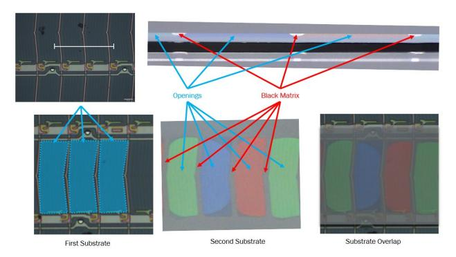
56. The Accused LCD Product has a second alignment film on the color filter substrate, as shown below.
