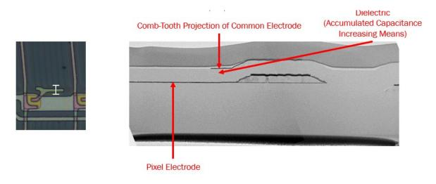
58. The Accused LCD Product has an active matrix type liquid crystal display device with an array substrate having a switching element array, an opposing substrate, and a liquid layer in between, as illustrated below in reference to K&D Technology LCD Model No. KD101N37-40NA-A10, shown below.
