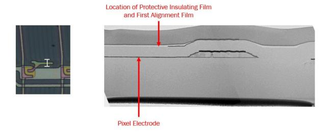
55. The Accused LCD Product has a second substrate with a black matrix with opening in areas opposite to the pixel electrodes, as shown below.
