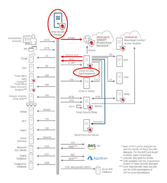
(See 12.0 Installation Guide at PDF p. 208.) As illustrated in this example, the Deep Security Manager receives data through the 4119 (or 443) and 4120 ports, and the Deep Security Agent/Agent and the Deep Security Manager send data to Trend Micro's Smart Protection network through 80/443 ports. (12.0 Installation Guide at 208.) Additionally, Trend Micro's Deep Security system allows the Deep Security Manager to "send events to an external Syslog or Security
