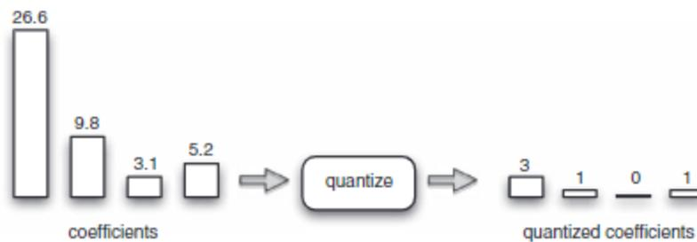
Figure 4.12 Quantization example
