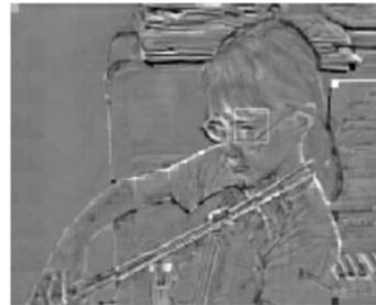
Figure 6.8 Residual after subtracting intra prediction
