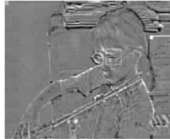
Figure 6.8 Residual after subtracting intra prediction
