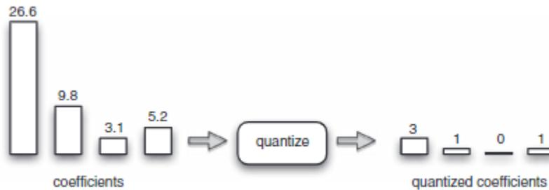
Figure 4.12 Quantization example
