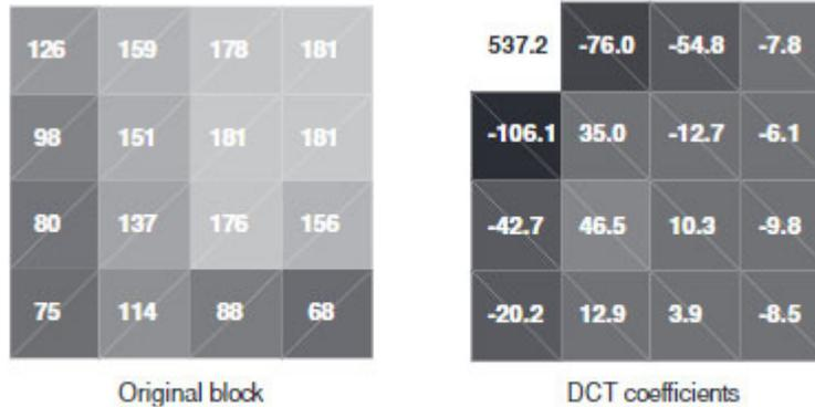
**Figure 3.31** Close-up of 4 × 4 block; DCT coefficients
