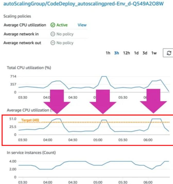
343. AWS Auto Scaling, in response to the detecting step, employs a system allocator to activate an additional server application on the server. For example, AWS Auto Scaling employs an auto scaling API to auto scale additional server application instances, depending on the AWS services utilized.<sup>163</sup>
