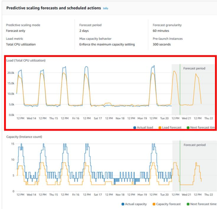
342. AWS Auto Scaling detects when the load exceeds an activation threshold. Auto Scaling groups in AWS Auto Scaling are configured to adhere to specified scaling metrics that detect when server load exceeds an activation threshold.<sup>162</sup>
