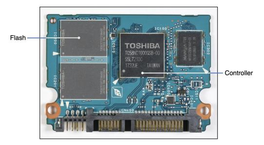
57. The Accused Products all contain a flash memory decoder comprising a decoding module configured to receive encoded data from flash memory. For example, on information and belief, the controller in the KSG60ZSE256G SSD includes a flash memory decoder comprising a decoding module configured to receive data with ECC encoding. As Kioxia has stated in a White
