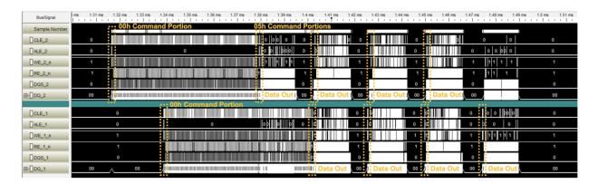
As shown above, each page read from flash memory is divided into four "chunks" of information bits and ECC bits. This is consistent with the ONFI ECC Codeword standard which recommends that "[t]he host transfers bytes from the page register in discrete units that include data, metadata, and the ECC check bytes."<sup>17</sup>
