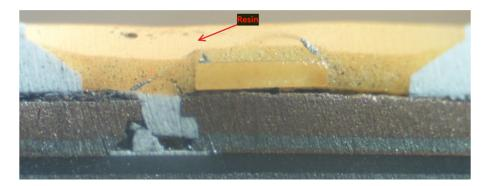
the example LED from the Globe 5"/6" Retrofit Smart Kit with the resin identified:
