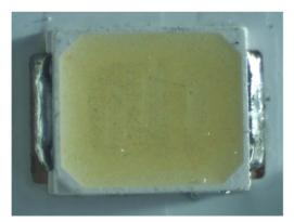
*1(b): a light-emitting element;*— The Ace Hardware A19 75W 5000k Bulb and Ace Hardware A19 100W 5000k Bulb each comprise a light-emitting element.
