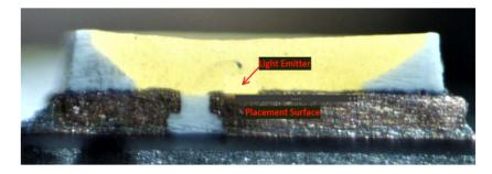
1(d): a transparent sealing resin that seals the light emitter, and forms a concave surface that is a light-outgoing surface via which light outgoes,— The Ace Hardware A19 60W 5000k Bulb and the Globe 5"/6" Retrofit Smart Kit each comprises a transparent sealing resin that seals the light emitter, and forms a concave surface that is a light-outgoing surface via which light outgoes.
