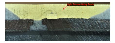
As another example, shown below is the cross-sectional view of the LED from the Ace Hardware LED Worklight with the light transmitting resin formed on the light emitting element and first and second lead frames identified:
