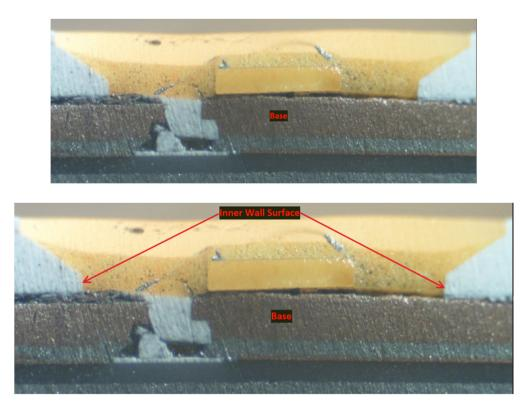
*1(c): a LED chip disposed on the inner bottom of the recess;*— The Ace Hardware A19 60W 5000k Bulb and the Globe 5"/6" Retrofit Smart Kit each comprise a LED chip disposed on the inner bottom of the recess.
