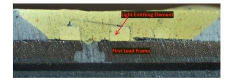
*1(d): a resin portion for fixing said first lead frame, said resin portion has a reflecting portion reflecting light emitted from said light-emitting element; and*— The Ace Hardware A19 75W 5000k Bulb and Ace Hardware A19 100W 5000k Bulb each comprise a resin portion for fixing said first lead frame, said resin portion has a reflecting portion reflecting light emitted from said light-emitting element.
