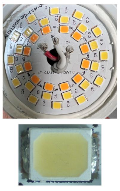
1(b): an LED chip;— The Ace Hardware A19 75W 2700k Bulb and the Globe A19 60WDuo Bright Bulb each comprise an LED chip.
