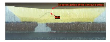
As another example, shown below is a cross sectional view of the LED from the Globe 5"/6" Retrofit Smart Kit with the light emitter and the electrode connected via a wire that is curved in such a way that a top section of the curved wire substantially coincides with a deepest section of the concave surface:
