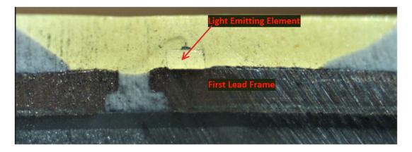
As another example, shown below is a resulting cross-sectional view of one crosssectioned LED chip from the Ace Hardware A19 100W 5000k Bulb with a first lead frame having a main surface on which the light-emitting element is mounted identified:
