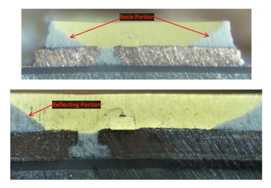
As another example, shown below is a cross-sectional view of the phosphor LED chip from the Ace Hardware A19 100W 5000k Bulb showing the resin portion for fixing the first lead frame, and the reflecting portion reflecting light from the light-emitting element:
