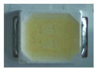
As another example, top-down views of an example semiconductor light-emitting apparatus from a Globe 5"/6" Retrofit Smart Kit are shown below:
