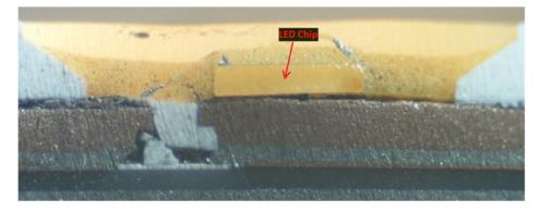
*1(d): a resin filled in the recess, the resin including phosphors which absorb a part of light emitted from the LED chip to convert the wavelength thereof and emit light;* — The Ace Hardware A19 60W 5000k Bulb and the Globe 5"/6" Retrofit Smart Kit each comprise a resin filled in the recess, the resin including phosphors which absorb a part of light emitted from the LED chip to convert the wavelength thereof and emit light.
