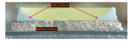
As another example, shown below is the cross-sectional view of the LED from the Ace Hardware LED Worklight with the light shielding resin covering a bottom surface and a side surface of the holding portion identified:
