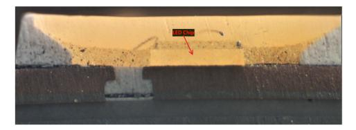
As another example, shown below is the cross-sectional view of the example phosphor LED from the Globe 5"/6" Retrofit Smart Kit with the LED chip identified:
