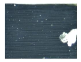
As another example, a face of the reflector formed into a rough surface is shown in the below image of the Ace Hardware LED Worklight:
