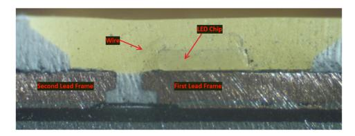
*1(e): a resin portion surrounding a circumference of said LED chip, and fastening said first and second lead frames,*— The Ace Hardware A19 75W 2700k Bulb and the Globe A19 60W Duo Bright Bulb each comprises a resin portion surrounding the circumference of the LED chip and fastening the first and second lead frames.
