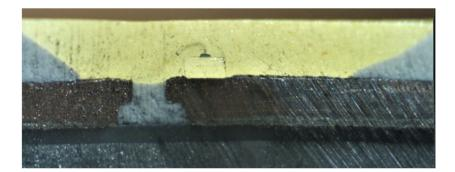
As another example, as shown below, the light shielding resin of the Ace Hardware LED Worklight is opaque, whereas the light transmitting resin is largely transparent. Accordingly, on information and belief, the light shielding resin of the Ace Hardware LED Worklight reflects a greater amount of light than the light transmitting resin.
