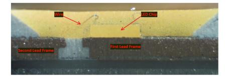
As another example, shown below are cross-sectional views of the cross-sectioned LED chip from the Globe A19 60W Duo Bright Bulb with a second lead frame electrically connected to the LED chip via a wire identified:
