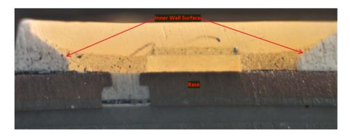
As another example, shown below are top-down and cross-sectional views of the example phosphor LED from the Globe 5"/6" Retrofit Smart Kit identifying a base with the upper surface opened, and the inner wall surface of the recess constituting a reflection surface identified in red:
