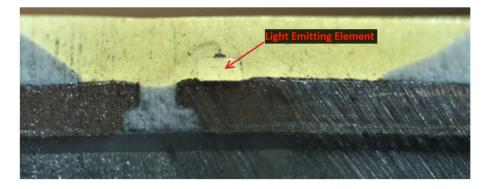
As another example, a cross section of an LED from the Ace Hardware LED Worklight was taken, and a resulting cross-sectional view is shown below with a semiconductor light emitting element identified:
