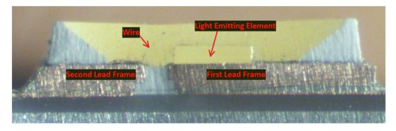
1(e): light transmitting resin formed on said semiconductor light emitting element and on said first and second lead frames,— The Ace Hardware A19 75W 5000k Bulb and the Ace
