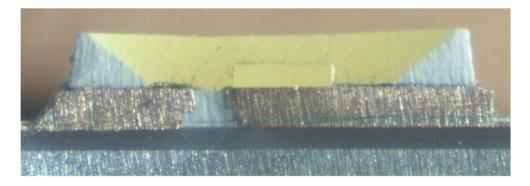
*1(h): wherein said light shielding resin is formed to cover a bottom surface and a side surface of said holding portion provided in said light transmitting resin.* — In the Ace Hardware A19 75W 5000k Bulb and the Ace Hardware LED Worklight, the light shielding resin is formed to cover a bottom surface and a side surface of the holding portion provided in the light transmitting resin.
