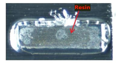
As another example, shown below is a top-down view of the example LED from the Ace Hardware LED Worklight with the LED removed and the resin disposed between the light emitting element identified:
