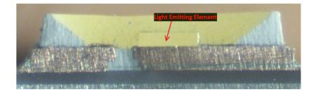
*1(d): a reflector on the substrate for reflecting a light beam outgoing from the light emitting element; and*— The Ace Hardware A19 2700k 75W Bulb, and the Ace Hardware LED Worklight each comprise a reflector on the substrate for reflecting a light beam outgoing from the light emitting element.
