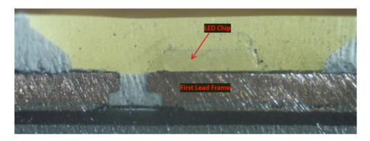
*1(d): a second lead frame electrically connected to said LED chip via a wire, and* — The Ace Hardware A19 75W 2700k Bulb and the Globe A19 60W Duo Bright Bulb each comprises a second lead frame that is electrically connected to the LED chip via a wire.
