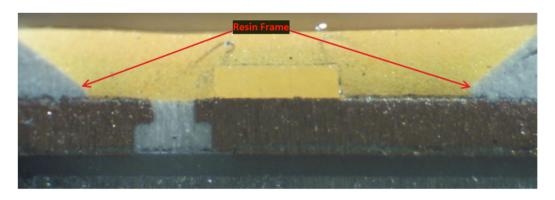
As another example, shown below is a cross-sectional view of a LED chip from the Globe A19 60W Duo Bright Bulb with a resin portion surrounding the circumference of the LED chip and fastening first and second lead frames identified:
