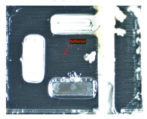
As another example, shown below is a top-down view of a phosphor LED from the Ace Hardware LED Worklight with the phosphor layer removed and the reflector identified:
