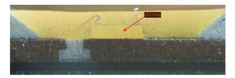
As another example, shown below are a top-down view and a cross-sectional view of the phosphor LED from the Globe A19 60W Duo Bright Bulb, respectively:
