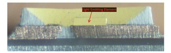
1(c): a first lead frame on which said semiconductor light emitting element is mounted;— The Ace Hardware A19 75W 5000k Bulb and the Ace Hardware LED Worklight each comprise a first lead frame on which said semiconductor light emitting element is mounted.
