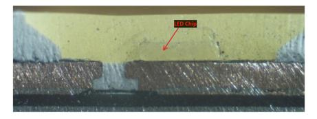
*1(c): a first lead frame on which said LED chip is mounted;*— The Ace Hardware A19 75W 2700k Bulb and the Globe A19 60W Duo Bright Bulb each comprise a first lead frame on which said LED chip is mounted.
