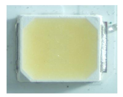
*1(b): a semiconductor light emitting element;*— The Ace Hardware A19 75W 5000k Bulb and the Ace Hardware LED Worklight each comprise a semiconductor light emitting element.
