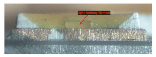
As another example, shown below is the cross-sectional view of the example phosphor LED from the Ace Hardware LED Worklight with the light emitting element on the substrate identified:
