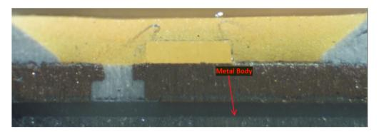
As another example, this configuration is shown in the below cross-sectional view of a cross-sectioned LED chip from the Globe A19 60W Duo Bright Bulb:
