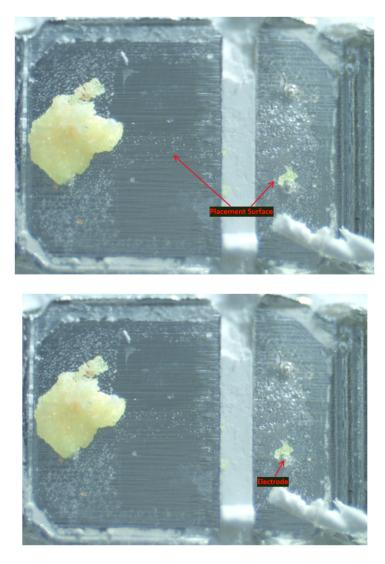
As another example, shown below are top down views of an LED from the Globe 5"/6" Retrofit Smart Kit with a placement surface that includes an electrode identified:
