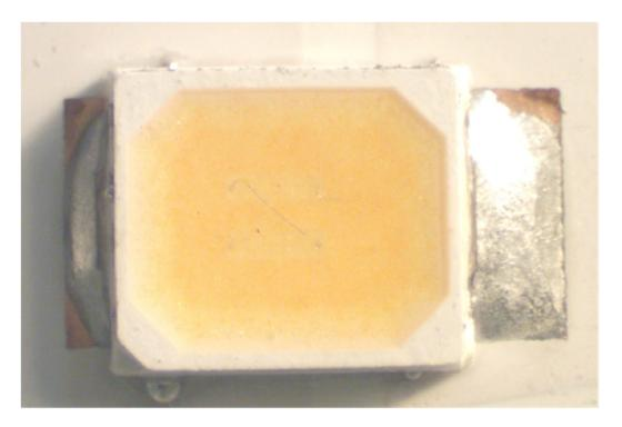
1(b): a base having a recess with the upper surface opened, the inner wall surface of the recess constituting a reflection surface;— The Ace Hardware A19 60W 5000k Bulb and the Globe 5"/6" Retrofit Smart Kit each comprise a base having a recess with the upper surface opened, the inner wall surface of the recess constituting a reflection surface.
