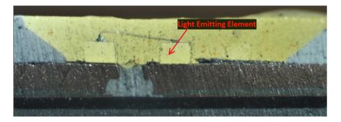
Hardware A19 100W 5000k Bulb with the light-emitting element identified:
