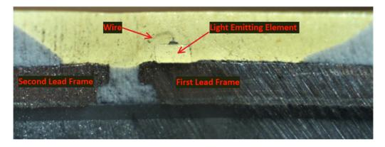
As another example, shown below are cross-sectional views of the phosphor LED chip from the Ace Hardware LED Worklight with the second lead frame electrically connected to the semiconductor light emitting element via a wire identified:
