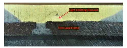
As another example, shown below is a resulting cross-sectional view of one crosssectioned LED chip from the Ace Hardware LED Worklight with a first lead frame having a main surface on which the light-emitting element is mounted:
