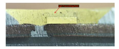
1(f): wherein said light emitting element is surrounded by a light shielding resin, wherein leading ends of said first and second lead frames are inserted into said light transmitting resin to provide a holding portion holding said first and second lead frames, — In the Ace Hardware A19 75W 5000k Bulb and the Ace Hardware LED Worklight, the light emitting element is surrounded by a light shielding resin, and leading ends of the first and second
