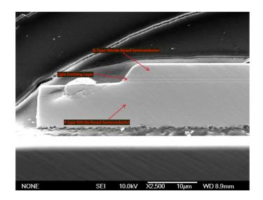
As another example, shown below is a close-up SEM image of the cross-sectioned LED chip from the Ikea Tradfri E26 LED Bulb identifying a p-type nitride-based semiconductor layer, a light emitting layer, and a n-type nitride-based semiconductor layer successively formed on the reflective layer:
