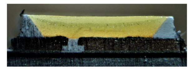
*1(h): wherein said light shielding resin is formed to cover a bottom surface and a side surface of said holding portion provided in said light transmitting resin.* — In the Ikea Maglehult LED light and the Ikea Ledare 5.5W E26 LED Bulb, the light shielding resin is formed to cover a bottom surface and a side surface of the holding portion provided in the light transmitting resin.
