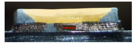
As another example, shown below is a cross-sectional view of an example phosphor LED from the Ikea Ryet G4 with the substrate annotated in red:
