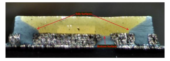
As another example, shown below is the cross-sectional view of the LED from the Ikea Ledare 5.5W E26 LED Bulb with the light shielding resin covering a bottom surface and a side surface of the holding portion identified:
