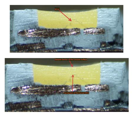
As another example, shown below is a cross sectional view of the LED from the Ikea Dioder LED light with the light emitter and the electrode connected via a wire that is curved in such a way that a top section of the curved wire substantially coincides with a deepest section of the concave surface:
