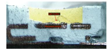
1(d): a transparent sealing resin that seals the light emitter, and forms a concave surface that is a light-outgoing surface via which light outgoes,— The Ikea Molgan and the
