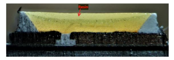
As another example, shown below is a close-up of a portion of the cross-sectional view of the example LED from the Ikea Ledare GX53 LED Bulb with the resin identified:
