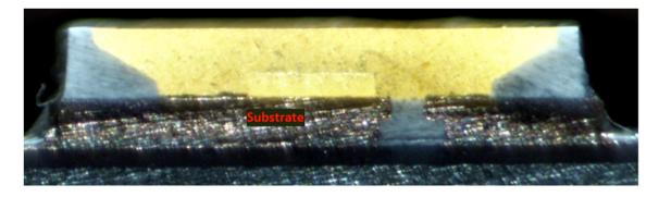
*1(c): a light emitting element on the substrate;*— The Ikea Ledare GX53 LED Bulb and the Ikea Ryet G4 each comprise a light emitting element on the substrate.
