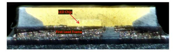
As another example, shown below is a resulting cross-sectional view of the one crosssectioned LED chip from the Ikea Ryet E12 LED Bulb with the one cross-sectioned LED chip mounted to a first lead frame identified:
