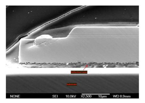
As a second example, the Ikea LEDberg Multicolor Lightstrip and the Ikea Tradfri E26 LED Bulb comprise a reflective layer formed on a support substrate.
