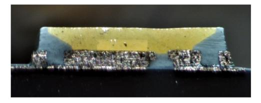
As another example, as shown below, the light shielding resin of the Ikea Ledare 5.5W E26 LED Bulb is opaque, whereas the light transmitting resin is largely transparent. Accordingly, on information and belief, the light shielding resin of the Ikea Ledare 5.5W E26 LED Bulb reflects a greater amount of light than the light transmitting resin.
