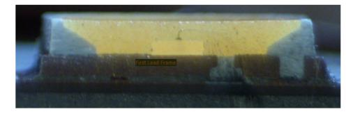
*I(d): a resin portion for fixing said first lead frame, said resin portion has a reflecting portion reflecting light emitted from said light-emitting element; and*— The Ikea Ryet E12 and the Ikea Ryet 1717G5 LED Bulb each comprise a resin portion for fixing said first lead frame, said resin portion has a reflecting portion reflecting light emitted from said light-emitting element.
