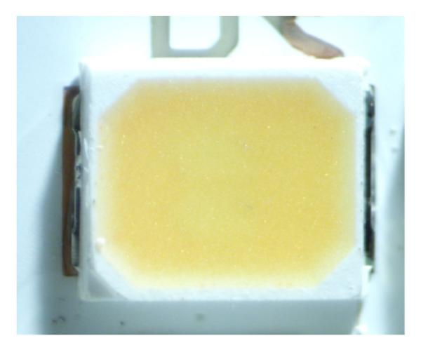
As another non-limiting example, the Ikea Ledare GX53 LED Bulb comprises a "light emitting device," as recited in claim 1.
