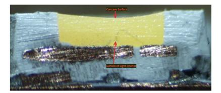
As another example, shown below is a cross-sectional view of the LED from the Ikea Dioder LED light with the concave surface facing a surface of the light emitter identified:
