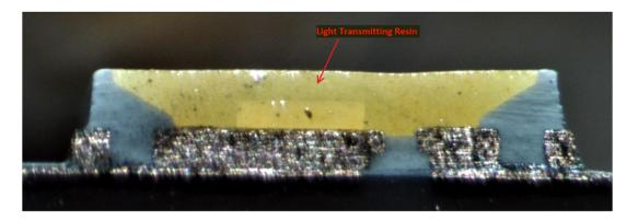
As another example, shown below is the cross-sectional view of the LED from the Ikea Ledare 5.5W E26 LED Bulb with the light transmitting resin formed on the light emitting element and first and second lead frames identified:
