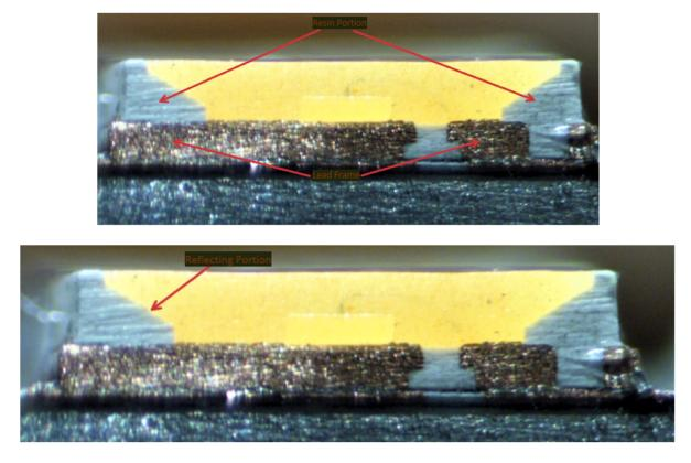
As another example, shown below is a cross-sectional view of the phosphor LED chip from the Ikea Ryet 1717G5 LED Bulb showing the resin portion for fixing the first lead frame, and the reflecting portion reflecting light from the light-emitting element:
