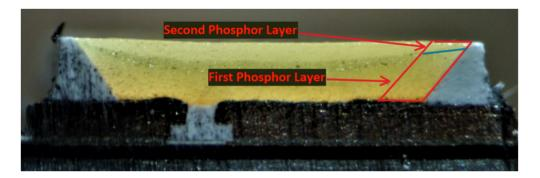
As shown above, the phosphor layer comprises a plurality of phosphor layers (*e.g.*, a first phosphor layer and a second phosphor layer) each of which is excited to emit a different wavelength of light from each other.
