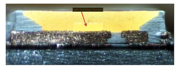
As another example, shown below is a cross-sectional view of the LED from the Ikea Ryet 1717G5 LED Bulb with the light-emitting element identified:
