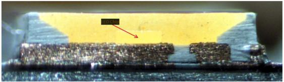
1(c): a first lead frame on which said LED chip is mounted;— The Ikea Ryet G4 and the Ikea Ryet E12 LED Bulb each comprise a first lead frame on which said LED chip is mounted.
