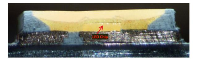
*I(d): a resin filled in the recess, the resin including phosphors which absorb a part of light emitted from the LED chip to convert the wavelength thereof and emit light*; — The Ikea Ledare 5.5W E26 and the Ikea Ledare GX53 LED Bulb each comprise a resin filled in the recess, the resin including phosphors which absorb a part of light emitted from the LED chip to convert the wavelength thereof and emit light.
