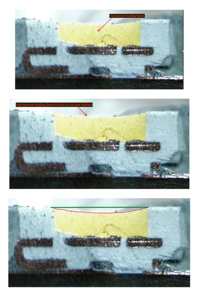
As shown above, the formed concave surface is a light-outgoing surface through which light outgoes.
