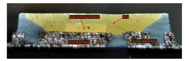
As another example, shown below are cross-sectional views of the phosphor LED chip from the Ikea Ledare 5.5W E26 LED Bulb with the second lead frame electrically connected to the semiconductor light emitting element via a wire identified:
