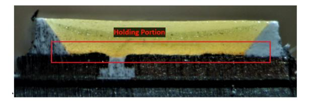
*I(g): wherein said light shielding resin has a reflectance higher than a reflectance of said light transmitting resin, and* — In the Ikea Maglehult LED light and the Ikea Ledare 5.5W E26 LED Bulb, the light shielding resin has a reflectance higher than a reflectance of the light transmitting resin.
