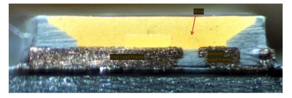
1(e): a resin portion surrounding a circumference of said LED chip, and fastening said first and second lead frames,— The Ikea Ryet G4 and the Ikea Ryet E12 LED Bulb each comprises a resin portion surrounding the circumference of the LED chip and fastening the first and second lead frames.
