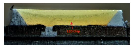
As another example, shown below is the cross-sectional view of the example phosphor LED from the Ikea Ledare GX53 LED Bulb with the LED chip identified:
