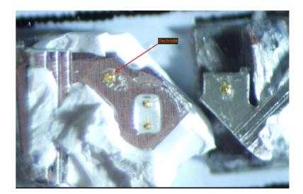
As another example, shown below are top down views of an LED from the Ikea Dioder LED light with a placement surface that includes an electrode identified:
