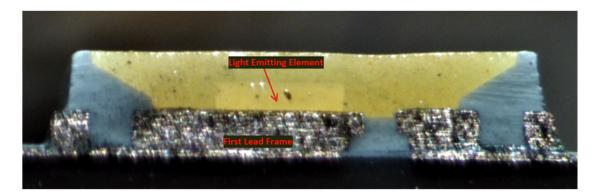
As another example, shown below is a resulting cross-sectional view of one crosssectioned LED chip from the Ikea Ledare 5.5W E26 LED Bulb with a first lead frame having a main surface on which the light-emitting element is mounted:
