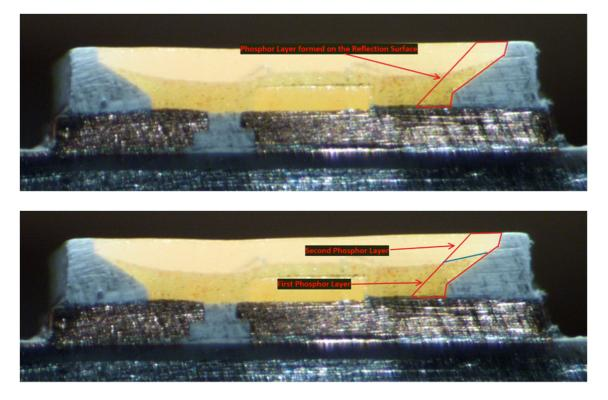
As shown above, the phosphor layer comprises a plurality of phosphor layers (*e.g.*, a first phosphor layer and a second phosphor layer) each of which is excited to emit a different wavelength of light from each other.
