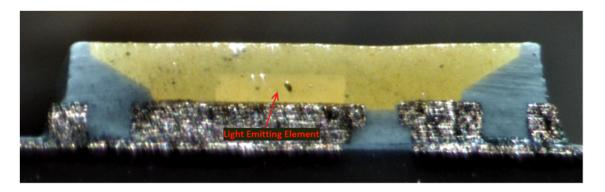
As another example, a cross section of an LED from a Ikea Ledare 5.5W E26 LED Bulb was taken, and a resulting cross-sectional view is shown below with a semiconductor light emitting element identified:
