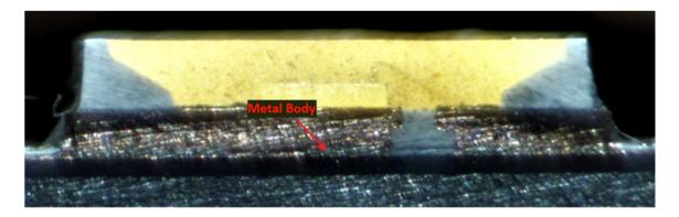
As another example, this configuration is shown in the below cross-sectional view of a cross-sectioned LED chip from the Ikea Ryet E12 LED Bulb:
