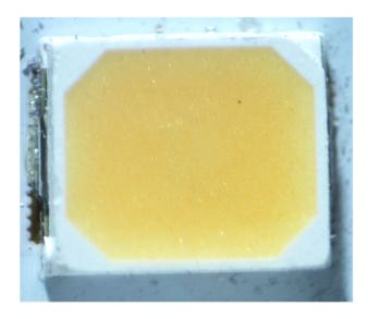
*1(b): an LED chip;*— The Ikea Ryet G4 and the Ikea Ryet E12 LED Bulb each comprise an LED chip.
