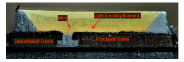
*1(e): light transmitting resin formed on said semiconductor light emitting element and on said first and second lead frames,*— The Ikea Maglehult LED light and the Ikea Ledare 5.5W E26 LED Bulb each comprise a light transmitting resin formed on said semiconductor light emitting element and on said first and second lead frames.
