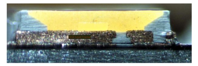
As another example, shown below is a resulting cross-sectional view of one crosssectioned LED chip from the Ikea Ryet 1717G5 LED Bulb with a first lead frame having a main surface on which the light-emitting element is mounted identified:
