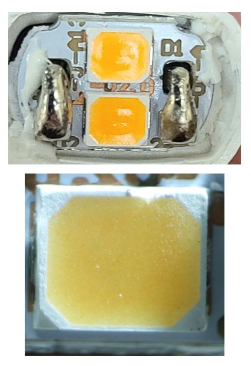
As another non-limiting example, the Ikea Ryet E12 LED Bulb comprises a "semiconductor light emitting device," as recited in claim 1.
