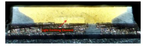
*1(d): a reflector on the substrate for reflecting a light beam outgoing from the light emitting element; and*— The Ikea Ledare GX53 LED Bulb and the Ikea Ryet G4 each comprise a reflector on the substrate for reflecting a light beam outgoing from the light emitting element.
