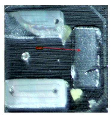
As another example, shown below is a top-down view of the example LED from the Ikea Ryet G4 with the LED removed and the resin disposed between the light emitting element identified:
