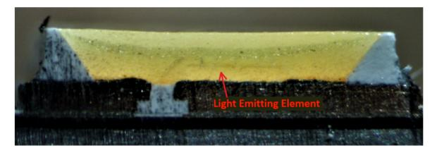
1(c): a first lead frame on which said semiconductor light emitting element is mounted;— The Ikea Maglehult LED light and the Ikea Ledare 5.5W E26 LED Bulb each comprise a first lead frame on which said semiconductor light emitting element is mounted.
