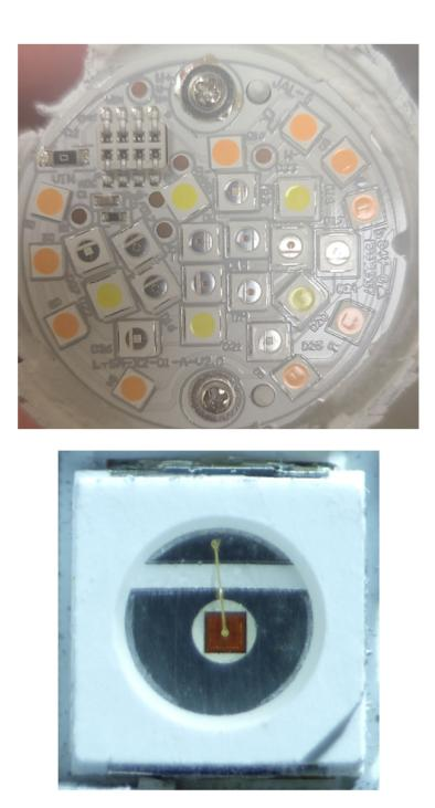
*1(b): a reflective layer formed on a support substrate;*— The Ikea LEDberg Multicolor Lightstrip and the Ikea Tradfri E26 LED Bulb comprise a reflective layer formed on a support substrate.
