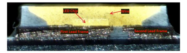
As another example, shown below are cross-sectional views of the cross-sectioned LED chip from the Ikea Ryet E12 LED Bulb with a second lead frame electrically connected to the LED chip via a wire identified:
