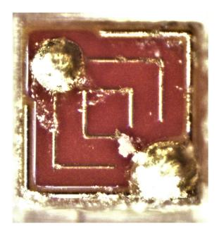
As another example, shown below are top views of a diode in the Ikea Tradfri E26 LED Bulb that shows a light extracting surface located above the n-type nitride-based semiconductor layer (shown above with respect to claim element 1(c)) having surface irregularities:
