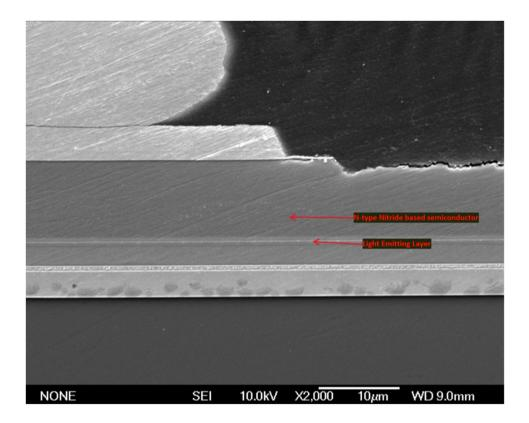
*1(d): wherein a light extracting surface located above said n-type nitride-based semiconductor layer has irregularities; and*— The Ikea LEDberg Multicolor Lightstrip and the Ikea Tradfri E26 LED Bulb comprise a light extracting surface that is located above the n-type nitride-based semiconductor layer and has irregularities.
