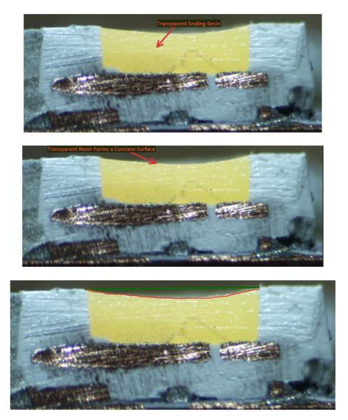
As shown above, the formed concave surface is a light-outgoing surface through which light outgoes.
