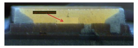
1(c): a first lead frame having a main surface having said light-emitting element mounted thereon;— The Ikea Ryet E12 and the Ikea Ryet 1717G5 LED Bulb each comprise a first lead frame having a main surface having said light-emitting element mounted thereon.
