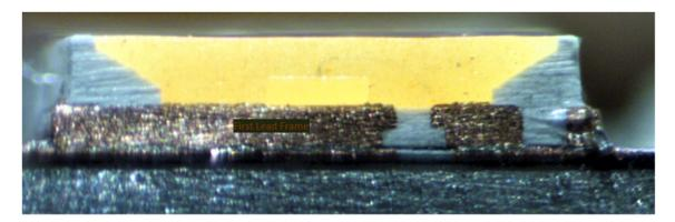
*1(d): a second lead frame electrically connected to said LED chip via a wire, and* — The Ikea Ryet G4 and the Ikea Ryet E12 LED Bulb each comprises a second lead frame that is electrically connected to the LED chip via a wire.
