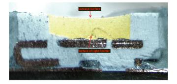
1(f): the light emitter and the electrode being connected via a wire that is curved in such a way that a top section of the curved wire substantially coincides with a deepest section of the concave surface,— The Ikea Molgan and the Ikea Dioder LED light each includes a light emitter and the electrode being connected via a wire that is curved in such a way that a top section of the curved wire substantially coincides with a deepest section.
