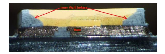
*1(c): a LED chip disposed on the inner bottom of the recess;*— The Ikea Ledare 5.5W E26 and the Ikea Ledare GX53 LED Bulb each comprise a LED chip disposed on the inner bottom of the recess.
