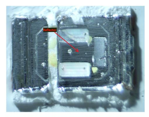
As another example, shown below is a top-down view of a phosphor LED from an Ikea Ryet G4 with the phosphor layer removed and the reflector identified:
