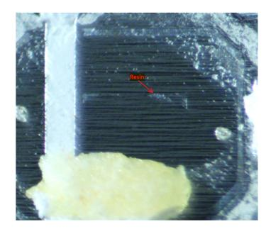
*1(f): wherein a face of the reflector on that reflects a light beam outgoing from the light emitting element is formed into a rough surface.*— In the Ikea Ledare GX53 LED Bulb and the Ikea Ryet G4, a face of the reflector that reflects a light beam outgoing from the light emitting element is formed into a rough surface.
