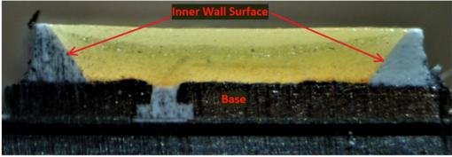
As another example, shown below are top-down and cross-sectional views of the example phosphor LED from the Ikea Ledare GX53 LED Bulb identifying a base with the upper surface opened, and the inner wall surface of the recess constituting a reflection surface identified in red:
