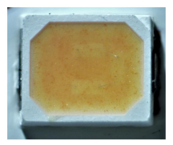
*1(b): a base having a recess with the upper surface opened, the inner wall surface of the recess constituting a reflection surface;*— The Ikea Ledare 5.5W E26 and the Ikea Ledare GX53 LED Bulb each comprise a base having a recess with the upper surface opened, the inner wall surface of the recess constituting a reflection surface.
