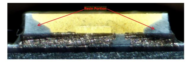
As another example, shown below is a cross-sectional view of a LED chip from an Ikea Ryet E12 LED Bulb with a resin portion surrounding the circumference of the LED chip and fastening first and second lead frames identified:
