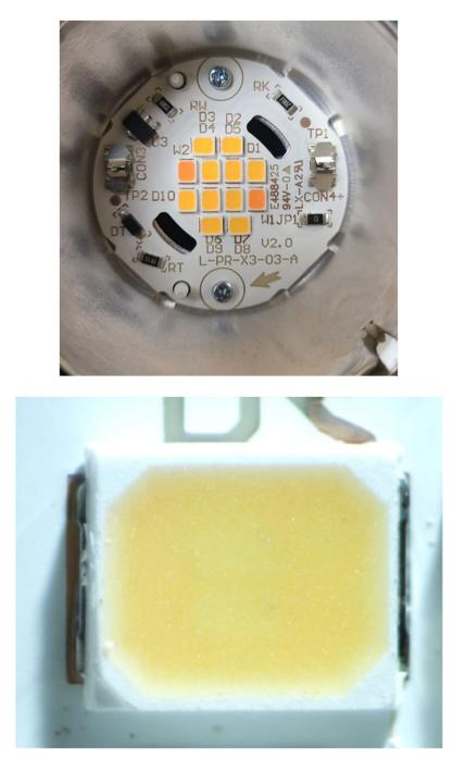
*1(b): a semiconductor light emitting element;*— The Ikea Maglehult LED light and the Ikea Ledare 5.5W E26 LED Bulb each comprise a semiconductor light emitting element.
