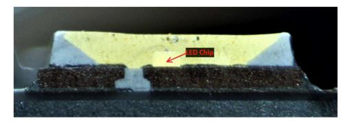
1(c): a first lead frame on which said LED chip is mounted;— The Target Up&Up 40W A19 Daylight Bulb and the Target Up&Up 60W A19 Daylight Bulb each comprise a first lead frame on which said LED chip is mounted.
