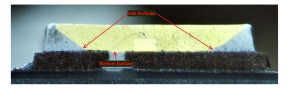
As another example, shown below is the cross-sectional view of the LED from the Target Up&Up 75W A19 Daylight Bulb with the light shielding resin covering a bottom surface and a side surface of the holding portion identified:
