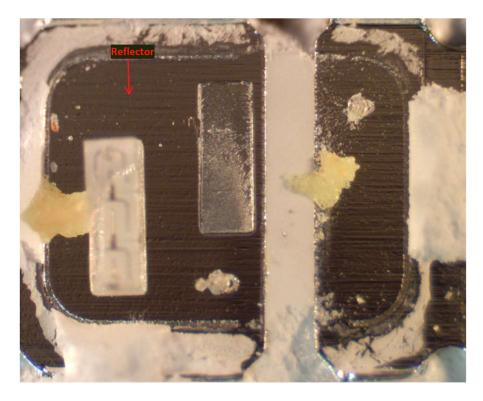
As another example, shown below is a top-down view of a phosphor LED from the Target Up&Up 90W Par38 Soft White Bulb with the phosphor layer removed and the reflector identified:
