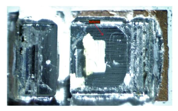
I(e): a resin disposed between the light emitting element and the reflector on the substrate,— The Target Up&Up 40W A19 Soft White Bulb and the Target Up&Up 90W Par38 Soft White Bulb each comprise a resin disposed between the light emitting element and the reflector on the substrate.
