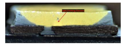
1(d): a reflector on the substrate for reflecting a light beam outgoing from the light emitting element; and— The Target Up&Up 40W A19 Soft White Bulb and the Target Up&Up 90W Par38 Soft White Bulb each comprise a reflector on the substrate for reflecting a light beam outgoing from the light emitting element.
