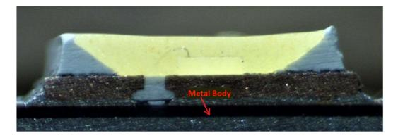
As another example, this configuration is shown in the below cross-sectional view of a cross-sectioned LED chip from the Target Up&Up 60W A19 Daylight Bulb:
