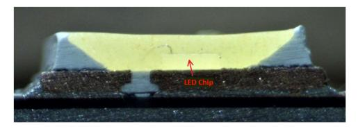
As another example, shown below are a top-down view and a cross-sectional view of the phosphor LED from the Target Up&Up 60W A19 Daylight Bulb, respectively:
