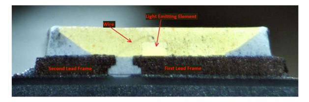
As another example, shown below are cross-sectional views of the phosphor LED chip from the Target Up&Up 75W A19 Daylight Bulb with the second lead frame electrically connected to the semiconductor light emitting element via a wire identified:
