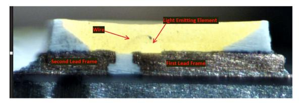
*I(e): light transmitting resin formed on said semiconductor light emitting element and on said first and second lead frames,*— The Target Up&Up 65W BR30 Daylight Bulb and the Target Up&Up 75W A19 Daylight Bulb each comprise a light transmitting resin formed on said semiconductor light emitting element and on said first and second lead frames.
