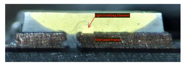
As another example, shown below is a resulting cross-sectional view of one cross-sectioned LED chip from the Target Up&Up 100W A19 Daylight Bulb with a first lead frame having a main surface on which the light-emitting element is mounted identified:
