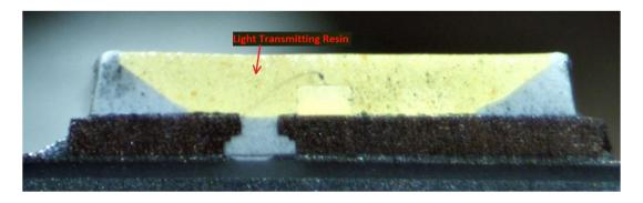
As another example, shown below is the cross-sectional view of the LED from the Target Up&Up 75W A19 Daylight Bulb with the light transmitting resin formed on the light emitting element and first and second lead frames identified:
