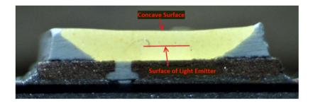
As another example, shown below is a cross-sectional view of the LED from the Target Up&Up 75W A19 Soft White Bulb with the concave surface facing a surface of the light emitter identified:
