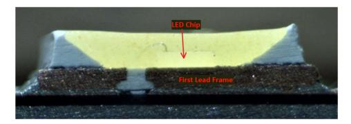
As another example, shown below is a resulting cross-sectional view of the one cross-sectioned LED chip from the Target Up&Up 60W A19 Daylight Bulb with the one cross-sectioned LED chip mounted to a first lead frame identified:
