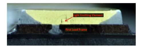
1(d): a resin portion for fixing said first lead frame, said resin portion has a reflecting portion reflecting light emitted from said light-emitting element; and— The Target Up&Up 90W Par38 Daylight Bulb and Target Up&Up 100W A19 Daylight Bulb each comprise a resin portion for fixing said first lead frame, said resin portion has a reflecting portion reflecting light emitted from said light-emitting element.
