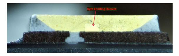
As another example, a cross section of an LED from the Target Up&Up 75W A19 Daylight Bulb was taken, and a resulting cross-sectional view is shown below with a semiconductor light emitting element identified:
