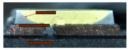
As shown above, the electrically-conductive layer is formed to extend from an area below the reflecting portion to the area outside the area covered by the reflecting portion.
