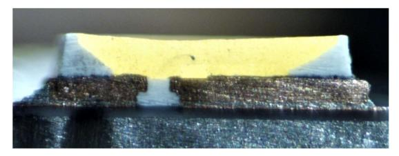
1(h): wherein said light shielding resin is formed to cover a bottom surface and a side surface of said holding portion provided in said light transmitting resin. — In the Target Up&Up 65W BR30 Daylight Bulb and the Target Up&Up 75W A19 Daylight Bulb, the light shielding resin is formed to cover a bottom surface and a side surface of the holding portion provided in the light transmitting resin.
