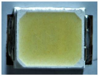
As another non-limiting example, the Target Up&Up 100W A19 Daylight Bulb comprises a "semiconductor light emitting device," as recited in claim 1.
