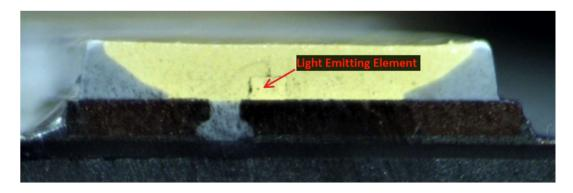
I(c): a first lead frame having a main surface having said light-emitting element mounted thereon;— The Target Up&Up 90W Par38 Daylight Bulb and Target Up&Up 100W A19 Daylight Bulb each comprise a first lead frame having a main surface having said light-emitting element mounted thereon.
