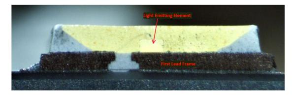
As another example, shown below is a resulting cross-sectional view of one cross-sectioned LED chip from the Target Up&Up 75W A19 Daylight Bulb with a first lead frame having a main surface on which the light-emitting element is mounted:
