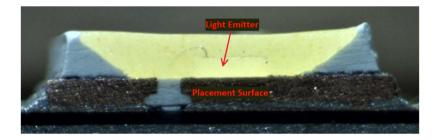
As another example, shown below is a cross-sectional view of the LED from the Target Up&Up 75W A19 Soft White Bulb with the light emitter placed on the placement surface identified:
