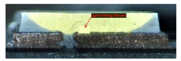
As another example, shown below is a cross-sectional view of the LED from the Target Up&Up 100W A19 Daylight Bulb with the light-emitting element identified:
