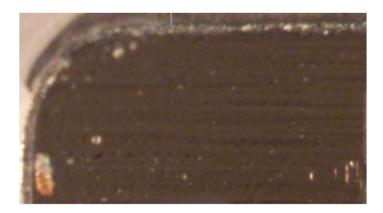
As another example, a face of the reflector formed into a rough surface is shown in the below image of the Target Up&Up 90W Par38 Soft White Bulb:
