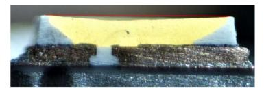
As shown above, the formed concave surface is a light-outgoing surface through which light outgoes.
