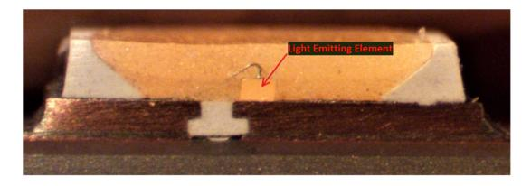
As another example, shown below is the cross-sectional view of the example phosphor LED from the Target Up&Up 90W Par38 Soft White Bulb with the light emitting element on the substrate identified:
