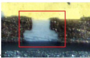
1(g): wherein said light shielding resin has a reflectance higher than a reflectance of said light transmitting resin, and — In the Target Up&Up 65W BR30 Daylight Bulb and the Target Up&Up 75W A19 Daylight Bulb, the light shielding resin has a reflectance higher than a reflectance of the light transmitting resin.
