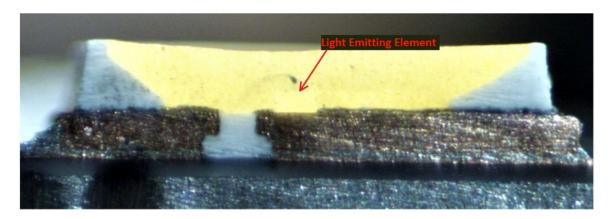
1(c): a first lead frame on which said semiconductor light emitting element is mounted;— The Target Up&Up 65W BR30 Daylight Bulb and the Target Up&Up 75W A19 Daylight Bulb each comprise a first lead frame on which said semiconductor light emitting element is mounted.
