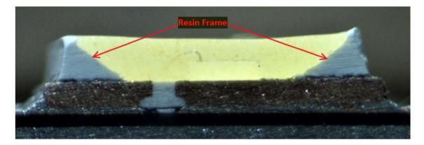
As another example, shown below is a cross-sectional view of a LED chip from the Target Up&Up 60W A19 Daylight Bulb with a resin portion surrounding the circumference of the LED chip and fastening first and second lead frames identified:
