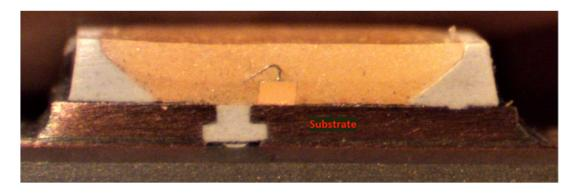
As another example, shown below is a cross-sectional view of an example phosphor LED from the Target Up&Up 90W Par38 Soft White Bulb with the substrate annotated in red:
