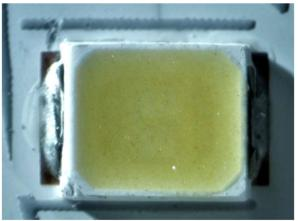
As another example, top-down views of an example semiconductor light-emitting apparatus from the Target Up&Up 75W A19 Soft White Bulb are shown below:
