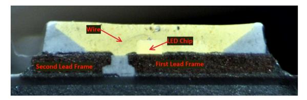
1(e): a resin portion surrounding a circumference of said LED chip, and fastening said first and second lead frames,— The Target Up&Up 40W A19 Daylight Bulb and the Target Up&Up 60W A19 Daylight Bulb each comprises a resin portion surrounding the circumference of the LED chip and fastening the first and second lead frames.
