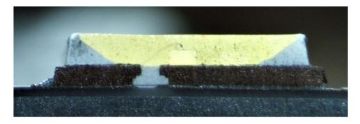
As another example, as shown below, the light shielding resin of the Target Up&Up 75W A19 Daylight Bulb is opaque, whereas the light transmitting resin is largely transparent. Accordingly, on information and belief, the light shielding resin of the Target Up&Up 75W A19 Daylight Bulb reflects a greater amount of light than the light transmitting resin.
