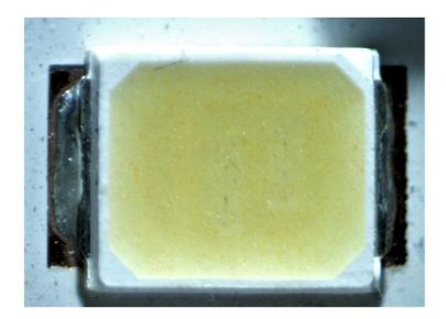
As another non-limiting example, the Target Up&Up 75W A19 Daylight Bulb comprises a "semiconductor light emitting device," as recited in claim 1.
