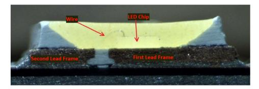
As another example, shown below are cross-sectional views of the cross-sectioned LED chip from the Target Up&Up 60W A19 Daylight Bulb with a second lead frame electrically connected to the LED chip via a wire identified:
