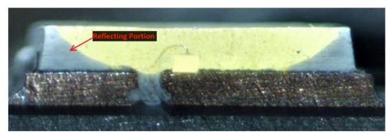
As another example, shown below is a cross-sectional view of the phosphor LED chip from the Target Up&Up 100W A19 Daylight Bulb showing the resin portion for fixing the first lead frame, and the reflecting portion reflecting light from the light-emitting element:
