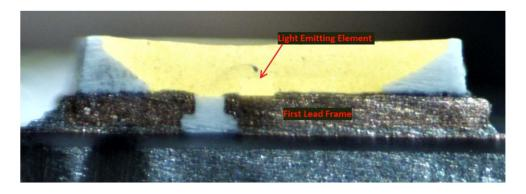
I(d): a second lead frame electrically connected to said semiconductor light emitting element via a wire,; and— The Target Up&Up 65W BR30 Daylight Bulb and the Target Up&Up 75W A19 Daylight Bulb each comprise a second lead frame electrically connected to said semiconductor light emitting element via a wire.
