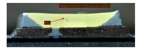
As another example, shown below is a cross sectional view of the LED from the Target Up&Up 75W A19 Soft White Bulb with the light emitter and the electrode connected via a wire that is curved in such a way that a top section of the curved wire substantially coincides with a deepest section of the concave surface:
