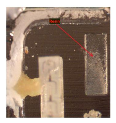
As another example, shown below is a top-down view of the example LED from the Target Up&Up 90W Par38 Soft White Bulb with the LED removed and the resin disposed between the light emitting element identified:
