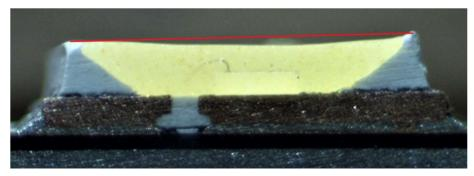
As shown above, the formed concave surface is a light-outgoing surface through which light outgoes.
