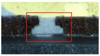
As another example, shown below is the cross-sectional view of the LED from the Target Up&Up 75W A19 Daylight Bulb with the light shielding resin and holding portion identified:
