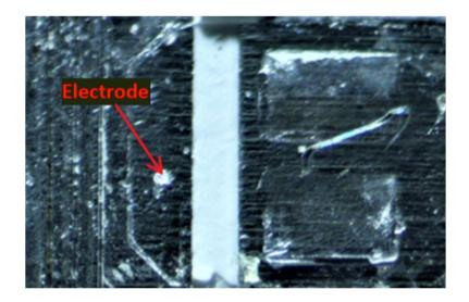
As another example, shown below are top down views of an LED from the Target Up&Up 75W A19 Soft White Bulb with a placement surface that includes an electrode identified:
