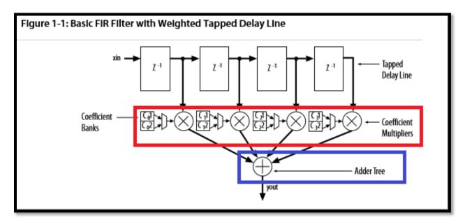
INTEL FIR II IP CORE USER GUIDE AT PAGE 4 (May 2016) (the red box identifies the coefficient multipliers that are added to the "adder tree" which is identified in the blue box).
