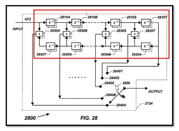
'166 PATENT, FIG. 28 (the red box annotation identifies the pre-addition unit in a figure of the '166 patent specification).
