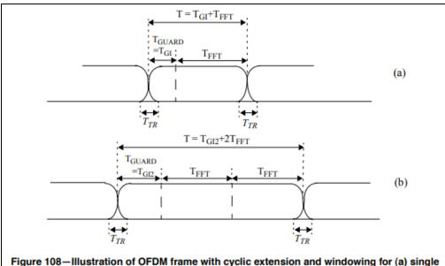
Figure 108—Illustration of OFDM frame with cyclic extension and windowing for (a) single reception or (b) two receptions of the FFT period
