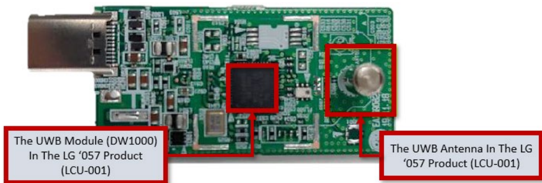
LG LCU-001 UWB MODULE TEARDOWN (annotation added).
