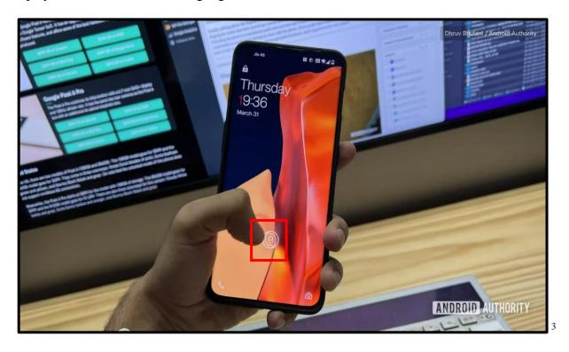
30. The OnePlus 10 Pro further comprises a sensing module integrated with the display
