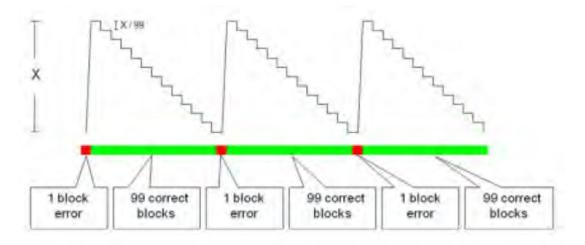
30. The convergence rate of the BLER is slow and potentially wastes significant potential code capacity within a RF channel. A more precise manner of adjusting the SIR<sub>Target</sub> is required. In the Qualcomm mobile transceivers incorporated into LG devices, a component is added to the SIR<sub>Target</sub> determination that accounts for the propagation of the channel for each code.
