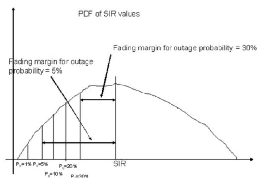
As shown in this figure, the Qualcomm mobile transceivers incorporated in the LG Accused Products calculate one or more outage probabilities as a percentage of the total sum of the SIR<sub>error</sub> values (under the curve, from minimum to maximum). Each outage probability can be calculated by maintaining the total sum of the SIR<sub>error</sub> values in the histogram and then summing
