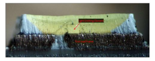
As another example, shown below is a resulting cross-sectional view of one crosssectioned LED chip from the Array by Hampton Full Color Smart A19 Bulb with a first lead frame having a main surface on which the light-emitting element is mounted identified:
