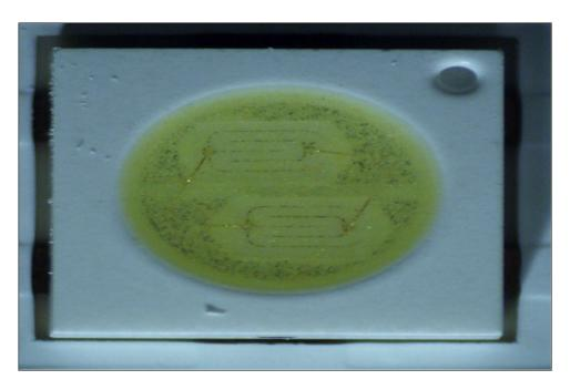
1(b): an LED chip;— The Array by Hampton Adjustable White Smart A19 Bulb and the Insignia NS-43DF710NA21 each comprise an LED chip.
