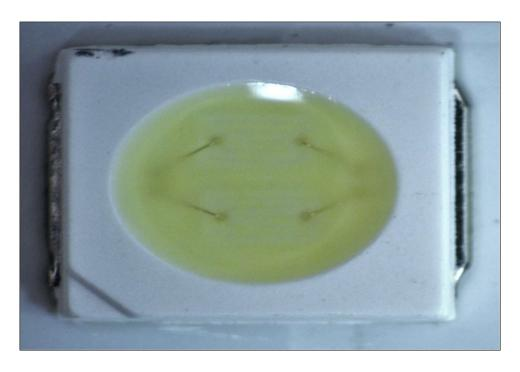
As another non-limiting example, the Array by Hampton Full Color Smart A19 Bulb comprises a "semiconductor light emitting device," as recited in claim 1.
