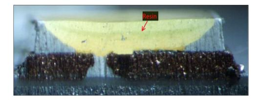
As another example, shown below is a close-up of a portion of the cross-sectional view of the example LED from the Array by Hampton Adjustable White Smart BR30 Bulb with the resin identified:
