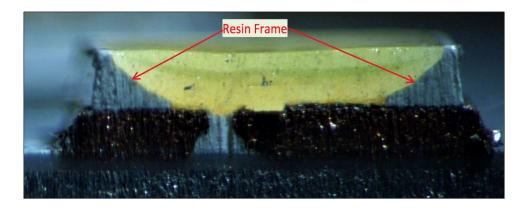
As another example, shown below is a cross-sectional view of a LED chip from an Insignia NS-43DF710NA21 with a resin portion surrounding the circumference of the LED chip and fastening first and second lead frames identified:
