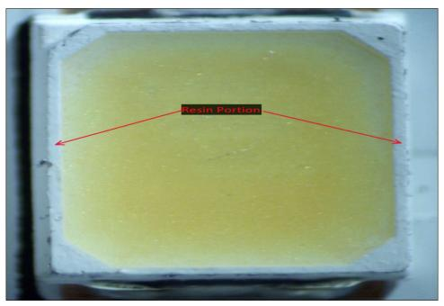
As another example, shown below is a cross-sectional view of the phosphor LED chip from the Array by Hampton Full Color Smart A19 Bulb showing the resin portion for fixing the first lead frame, and the reflecting portion reflecting light from the light-emitting element:
