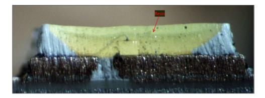
1(e): a phosphor layer formed on the reflection surface, the phosphor layer including the phosphors, wherein the phosphor layer comprises a plurality of phosphor layers each of which is excited to emit a different wavelength of light from each other,— The Array by Hampton Adjustable White Smart A19 Bulb and the Array by Hampton Adjustable White Smart BR30 Bulb each comprise a phosphor layer formed on the reflection surface, the phosphor layer including the phosphors, wherein
