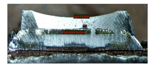
1(d): a transparent sealing resin that seals the light emitter, and forms a concave surface that is a light-outgoing surface via which light outgoes,— The Insignia NS-24DF310NA21 and the Array by Hampton Smart LED Strip each comprises a transparent sealing resin that seals the light emitter, and forms a concave surface that is a light-outgoing surface via which light outgoes.
