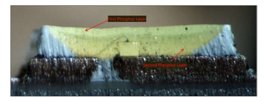
As shown above, the phosphor layer comprises a plurality of phosphor layers (e.g., a first phosphor layer and a second phosphor layer) each of which is excited to emit a different wavelength of light from each other.
