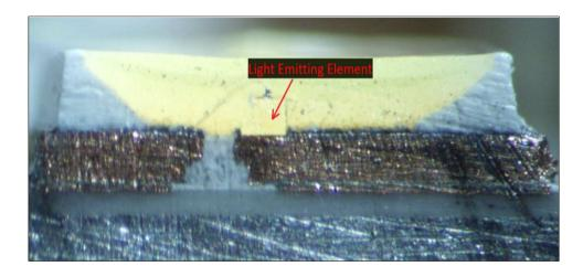
1(c): a first lead frame having a main surface having said light-emitting element mounted thereon;— The Array by Hampton Adjustable White Smart BR30 Bulb and the Array by Hampton Full Color Smart A19 Bulb each comprise a first lead frame having a main surface having said light-emitting element mounted thereon.
