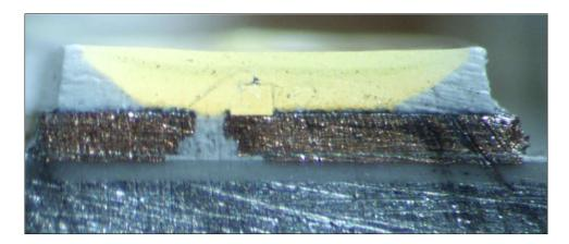
1(h): wherein said light shielding resin is formed to cover a bottom surface and a side surface of said holding portion provided in said light transmitting resin. — In the Insignia NS-24DF310NA21 and the Array by Hampton Full Color Smart A19 Bulb, the light shielding resin is formed to cover a bottom surface and a side surface of the holding portion provided in the light transmitting resin.
