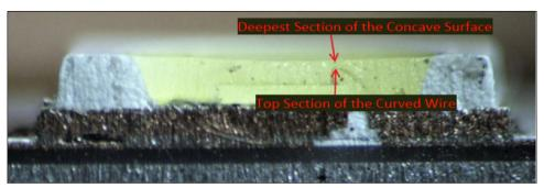
As another example, shown below is a cross sectional view of the LED from the Array by Hampton Smart LED Strip with the light emitter and the electrode connected via a wire that is curved in such a way that a top section of the curved wire substantially coincides with a deepest section of the concave surface:
