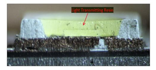
As another example, shown below is the cross-sectional view of the LED from the Array by Hampton Full Color Smart A19 Bulb with the light transmitting resin formed on the light emitting element and first and second lead frames identified:
