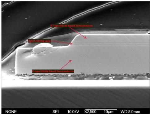
1(d): wherein a light extracting surface located above said n-type nitridebased semiconductor layer has irregularities; and— The Array by Hampton Smart
