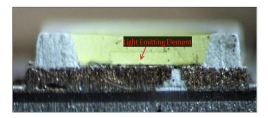
As another example, a cross section of an LED from an Array by Hampton Full Color Smart A19 Bulb was taken, and a resulting cross-sectional view is shown below with a semiconductor light emitting element identified:
