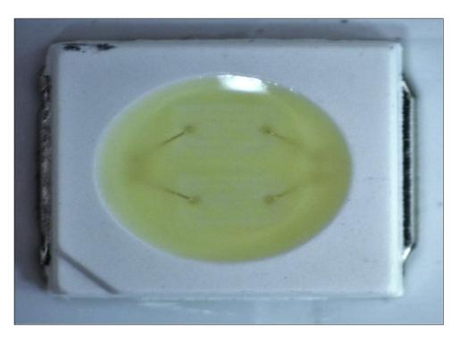
As another example, top-down views of an example semiconductor light-emitting apparatus from an Array by Hampton Smart LED Strip are shown below:
