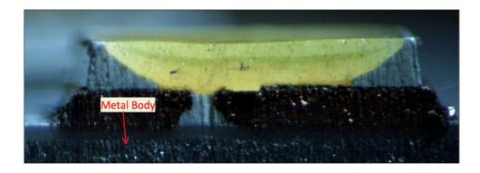
As another example, this configuration is shown in the below cross-sectional view of a cross-sectioned LED chip from the Insignia NS-43DF710NA21:
