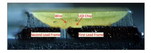
As another example, shown below are cross-sectional views of the cross-sectioned LED chip from the Insignia NS-43DF710NA21 with a second lead frame electrically connected to the LED chip via a wire identified:
