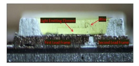
As another example, shown below are cross-sectional views of the phosphor LED chip from the Array by Hampton Full Color Smart A19 Bulb with the second lead frame electrically connected to the semiconductor light emitting element via a wire identified:
