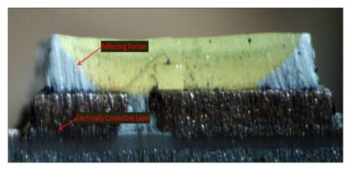
As shown above, the electrically-conductive layer is formed to extend from an area below the reflecting portion to the area outside the area covered by the reflecting portion.
