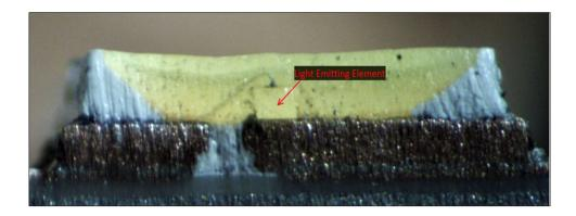
As another example, shown below is a cross-sectional view of the LED from the Array by Hampton Full Color Smart A19 Bulb with the light-emitting element identified:
