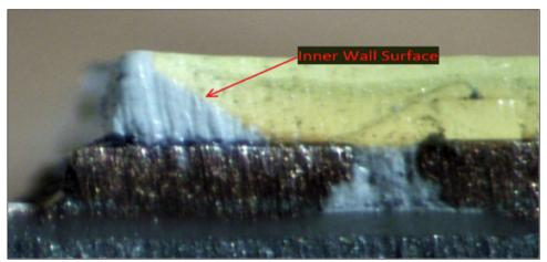
1(c): a LED chip disposed on the inner bottom of the recess;— The Array by Hampton Adjustable White Smart A19 Bulb and the Array by Hampton Adjustable White Smart BR30 Bulb each comprise a LED chip disposed on the inner bottom of the recess.
