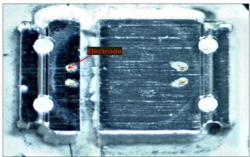
As another example, shown below are top down views of an LED from the Array by Hampton Smart LED Strip with a placement surface that includes an electrode identified:
