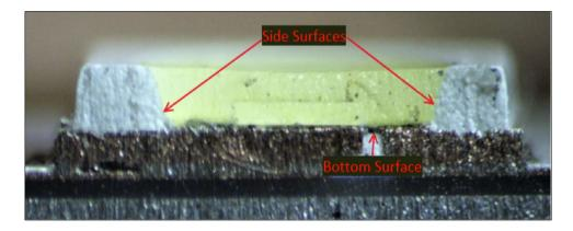
As another example, shown below is the cross-sectional view of the LED from the Array by Hampton Full Color Smart A19 Bulb with the light shielding resin covering a bottom surface and a side surface of the holding portion identified:
