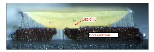
As another example, shown below is a resulting cross-sectional view of the one cross-sectioned LED chip from the Insignia NS-43DF710NA21 with the one cross-sectioned LED chip mounted to a first lead frame identified:
