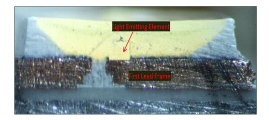
1(d): a resin portion for fixing said first lead frame, said resin portion has a reflecting portion reflecting light emitted from said light-emitting element; and— The Array by Hampton Adjustable White Smart BR30 Bulb and the Array by Hampton Full Color Smart A19 Bulb each comprise a resin portion for fixing said first lead frame, said resin portion has a reflecting portion reflecting light emitted from said light-emitting element.
