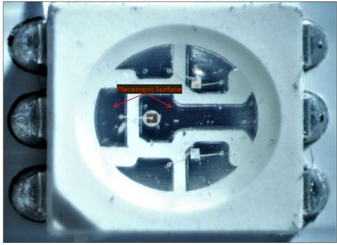
1(c): a light emitter that is placed on the placement surface;— The Insignia NS-24DF310NA21 and the Array by Hampton Smart LED Strip comprises a light emitter that is placed on the placement surface.
