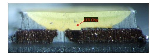
As another example, shown below is the cross-sectional view of the example phosphor LED from the Array by Hampton Adjustable White Smart BR30 Bulb with the LED chip identified:
