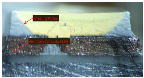
As shown above, the electrically-conductive layer is formed to extend from an area below the reflecting portion to the area outside the area covered by the reflecting portion.
