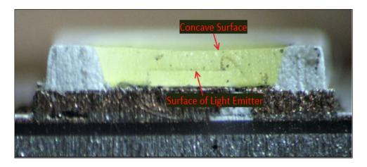
As another example, shown below is a cross-sectional view of the LED from the Array by Hampton Smart LED Strip with the concave surface facing a surface of the light emitter identified:
