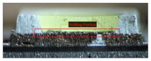
As another example, shown below is the cross-sectional view of the LED from the Array by Hampton Full Color Smart A19 Bulb with the light shielding resin and holding portion identified:
