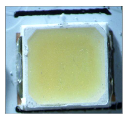
As another non-limiting example, the Array by Hampton Adjustable White Smart BR30 Bulb comprises a "light emitting device," as recited in claim 1.
