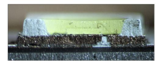
As another example, as shown below, the light shielding resin of the Array by Hampton Full Color Smart A19 Bulb is opaque, whereas the light transmitting resin is largely transparent. Accordingly, on information and belief, the light shielding resin of the Array by Hampton Full Color Smart A19 Bulb reflects a greater amount of light than the light transmitting resin.
