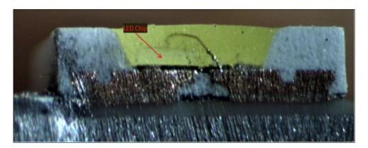
1(c): a first lead frame on which said LED chip is mounted;— The Array by Hampton Adjustable White Smart A19 Bulb and the Insignia NS-43DF710NA21 each comprise a first lead frame on which said LED chip is mounted.
