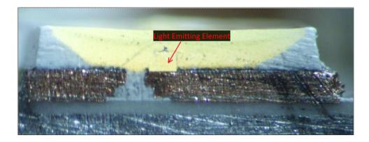
1(c): a first lead frame on which said semiconductor light emitting element is mounted;— The Insignia NS-24DF310NA21 and the Array by Hampton Full Color Smart A19 Bulb each comprise a first lead frame on which said semiconductor light emitting element is mounted.
