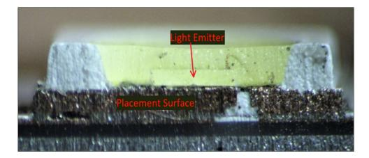
As another example, shown below is a cross-sectional view of the LED from the Array by Hampton Smart LED Strip with the light emitter placed on the placement surface identified:
