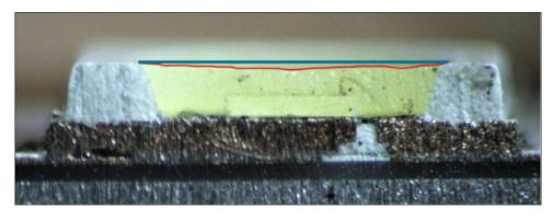
As shown above, the formed concave surface is a light-outgoing surface through which light outgoes.
