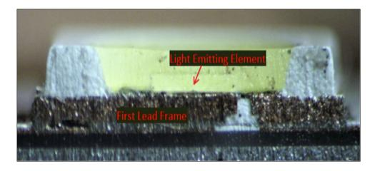
As another example, shown below is a resulting cross-sectional view of one cross-sectioned LED chip from the Array by Hampton Full Color Smart A19 Bulb with a first lead frame having a main surface on which the light-emitting element is mounted:
