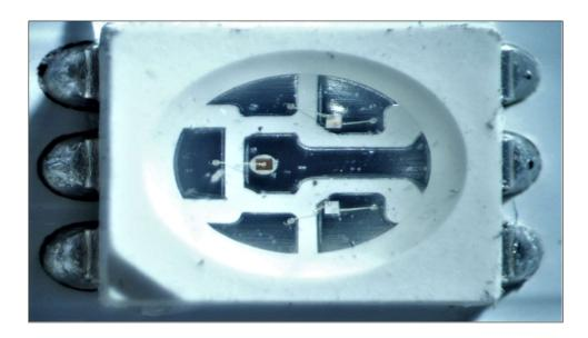
1(b): a placement surface that includes an electrode; — The Insignia NS-24DF310NA21 and the Array by Hampton Smart LED Strip comprises a placement surface that includes an electrode.
