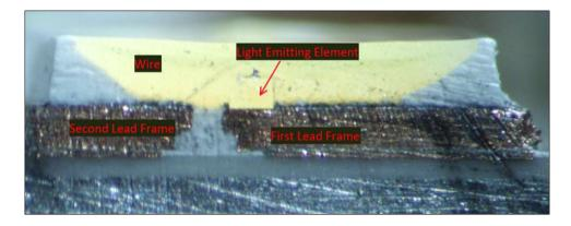
1(e): light transmitting resin formed on said semiconductor light emitting element and on said first and second lead frames,— The Insignia NS-24DF310NA21 and the Array by Hampton Full Color Smart A19 Bulb each comprise a light transmitting resin formed on said semiconductor light emitting element and on said first and second lead frames.
