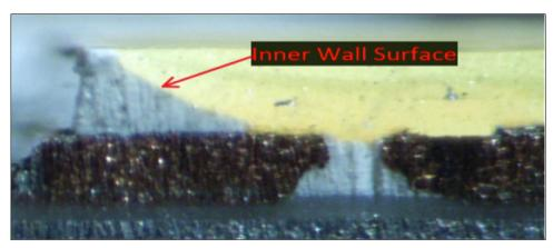
As another example, shown below are top-down and cross-sectional views of the example phosphor LED from the Array by Hampton Adjustable White Smart BR30 Bulb identifying a base with the upper surface opened, and the inner wall surface of the recess constituting a reflection surface identified in red:
