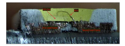
1(e): a resin portion surrounding a circumference of said LED chip, and fastening said first and second lead frames,— The Array by Hampton Adjustable White Smart A19 Bulb and the Insignia NS-43DF710NA21 each comprises a resin portion surrounding the circumference of the LED chip and fastening the first and second lead frames.
