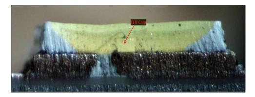
1(d): a resin filled in the recess, the resin including phosphors which absorb a part of light emitted from the LED chip to convert the wavelength thereof and emit light; — The Array by Hampton Adjustable White Smart A19 Bulb and the Array by Hampton Adjustable White Smart BR30 Bulb each comprise a resin filled in the recess, the resin including phosphors which absorb a part of light emitted from the LED chip to convert the wavelength thereof and emit light.
