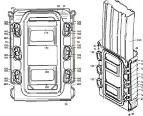
The claims of the '973 Patent are directed towards an expandable, variable compression pouch with an exoskeleton construction. As shown in the picture to the right, the hybrid construction combines a soft, flexible shell with semi-flexible molded outer components on the back, sides, bottom and front of the flexible shell. These molded components form an exoskeleton that provides structural reinforcement where needed without limiting the
