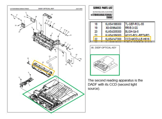
20. As shown below, the e-STUDIO5506AC printer is designed such that sheets of paper to be duplex scanned are placed in the ADF tray from which they are fed by rollers into the ADF. By design, during duplex scanning, the document is transported in a single direction by the rollers—from the ADF tray, the document page is moved past the surface of the flatbed scanner and then up into the ADF and past the ADF CCDM before being ejected into the ADF bin when scanning is complete. In
