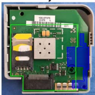
The ground plane (indicated in green) operates in cooperation with the radiating element
