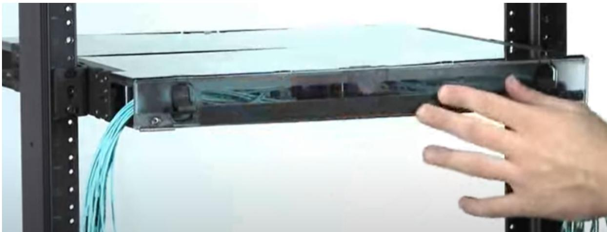
**FIG. 16.** Source: <https://www.youtube.com/watch?v=2fk-TIM8TOI> at 9:06 (view from front depicting the side cable access through the chassis after tray is in the closed position). (last visited November 9, 2022).
