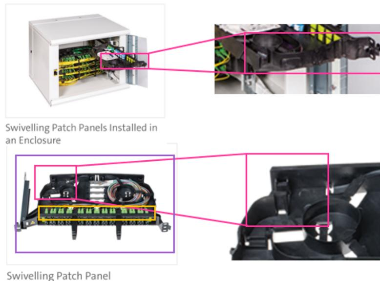
**FIG. 24.** Source: <https://www.corning.com/catalog/coc/documents/brochures/CRR-926-A4-BEN.pdf> (last visited November 9, 2022) (swiveling patch panel tray detail with cable entry/exit openings in pink and cable connection locations in yellow).
