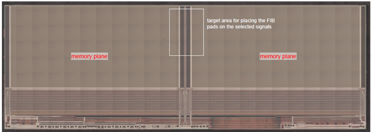
Toshiba 256 Gb 96L 3D NAND Flash Memory Die Photograph
