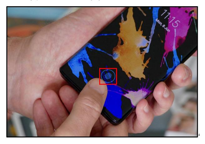
30. For example, the Motorola Edge further comprises a sensing module integrated with the display unit:
