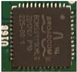
This exact same Power over Ethernet chip is incorporated into the products that Network-1 accused of infringing its '930 Patent and that were licensed. Broadcom witnesses were involved in the Network-1 trials asserting its '930 Patent. The data sheet and product materials for this BC M59111 Power over Ethernet chip (used in Defendant's products) were trial exhibits (P118
