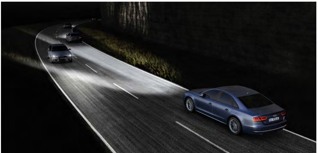
❶ With the glare-free all-time main beam in the Audi A8 either oncoming traffic or driving-in-front vehicles are precisely illuminated
