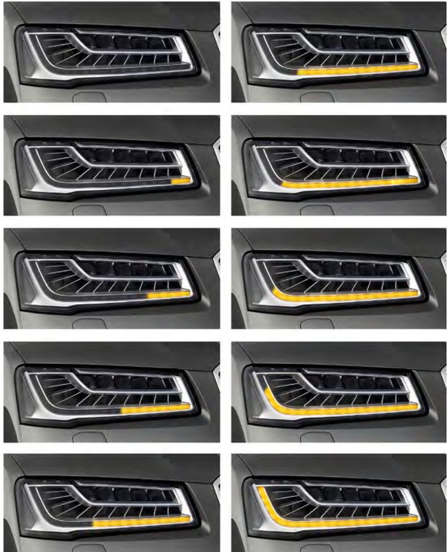
5 Temporal resolution of the dynamic LED turn indicator (picture sequence from top to down)
