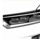
Up-Level System – Three LED Projectors (UWN)
