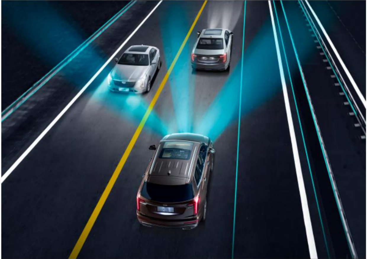
Cadillac XT6 headlamp– The adaptive matrix headlight system available on XT6 provides optimal lighting via intelligent adjustment of its 28 LED segments and cornering lamp functionality. Provided By General Motors
