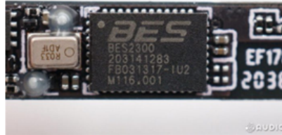
OnePlus Buds Z Bluetooth Audio Chip Bestechnic (BES) BES2300IU2
