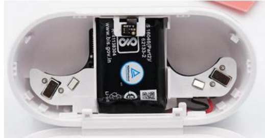
OnePlus Buds Z Base Station Motherboard (Charging Pins)
