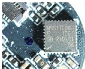
Nuvoton MS51TC0AE Microcontroller
