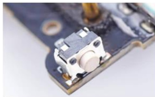
OnePlus Nord Buds Base Station Motherboard (Setup Button)
