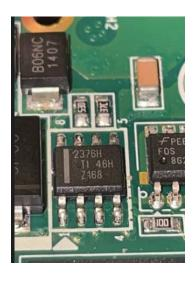
PoE products use Texas Instruments TPS chips to help execute the Power over Ethernet functionally in Defendant's products. In this picture of a circuit board from Defendant's PoE Camera, the Texas Instruction TP2376 Power over Ethernet chip is depicted in the center:
