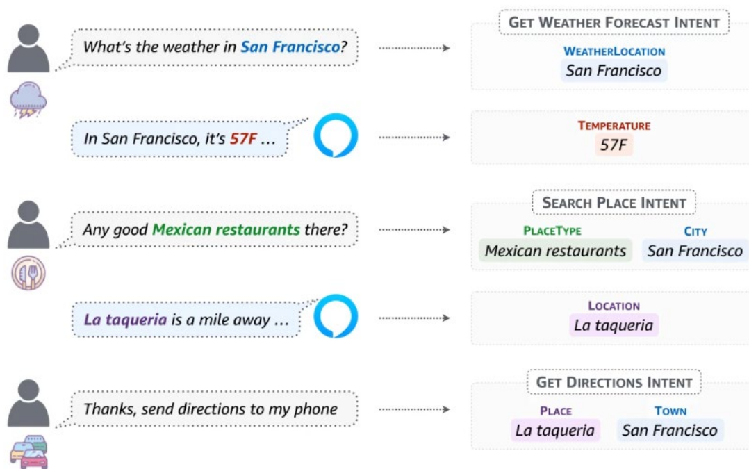
Different Alexa intents (weather, search, directions) might assign the same data (San Francisco) to different slots (WeatherLocation, City, Town). Tracking references by carrying slots over from one intent to the next is crucial for maintaining a coherent conversation.
