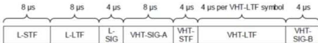
Figure 21-28—VHT NDP format
