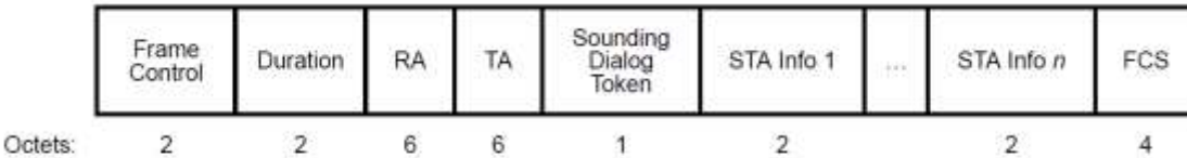
Figure 9-49—VHT NDP Announcement frame format
