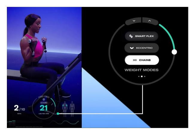
15. Tonal's dynamic weight modes also make workouts safer for its users. Tonal's "Spotter" and "Burnout" modes, for example, reduce resistance if a user is struggling or fatigued so that the user can complete a repetition or set without injury.
