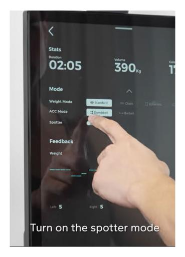
146. When the machine is in "Spotter" mode, the processor will instruct the motor to decrease the resistance provided to the cables when the user takes too long to complete the repetition<sup>41</sup>:
