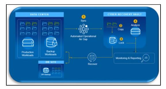
79. As explained by Dell, "the PowerProtect Cyber Recovery vault offers multiple layers of protection to provide resilience against cyberattacks even from an insider threat. It moves critical data away from the attack surface, physically isolating it within a protected part of the data center and requires separate security credentials and multi-factor authentication for access. Additional safeguards include an automated operational air gap to provide network isolation and eliminate management
