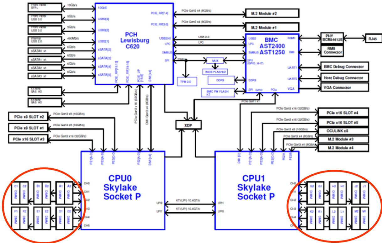
Figure 1: Motherboard Block Diagram
