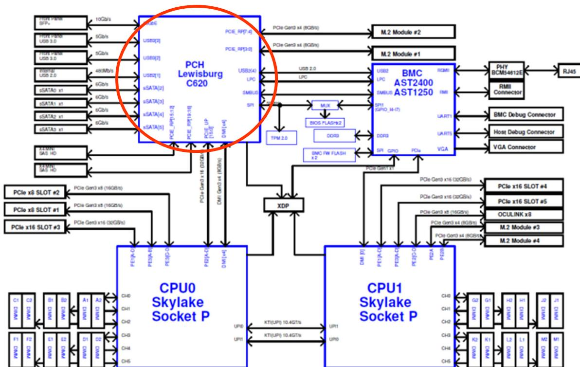
Figure 1: Motherboard Block Diagram
