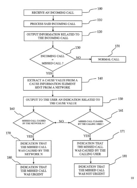
17. Figure 2 provides specific and detailed rules for the '872 patent's claimed call apparatus, making the invention concrete.
