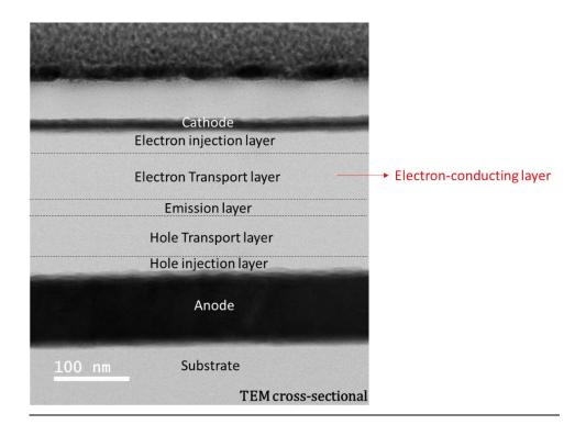
Moreover, on information and belief, "the electron-conducting layer is obtained by joint vaporization of a metal complex, which comprises a central metal atom," e.g., a lithium metal complex, such as the Liq compound shown below,
