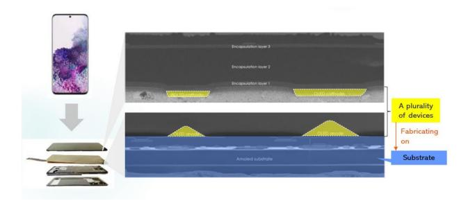
"selectively depositing at least one planarization layer upon said devices" and "selectively depositing at least one barrier layer over said planarization layer," as in an example shown below;
