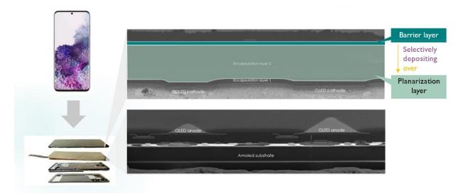
and wherein the planarization and barrier layers are selectively deposited (as shown in purple in the example below) without covering the edge, data driver, or camera hole (as shown in red in the example below).
