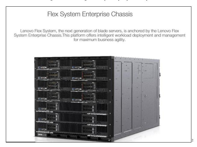
24. The Lenovo Flex System Enterprise Chassis further comprises a shroud coupled to said chassis to form an enclosure about said plurality of planar shaped circuit cards. The plurality of planar shaped circuit cards is each configured for providing an independent dedicated server
