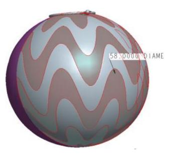
m. R12 Version (2021.7.17): Modified the method of magnet fixation. The magnet is embedded and molded as a single unit in the mold, with the magnet mold positioning hole on the surface of the sphere.
