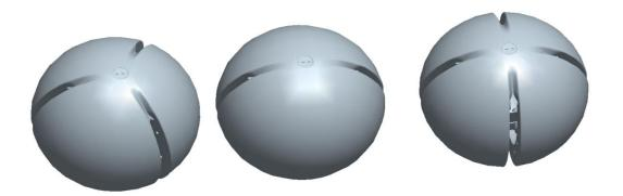
R3 Version (2020.11.26): Modified the mold shape of the water balloon body. Added sealing lips. The method of magnet fixation on PC plastic components was eliminated, and magnets were manually assembled onto the water balloon body.
