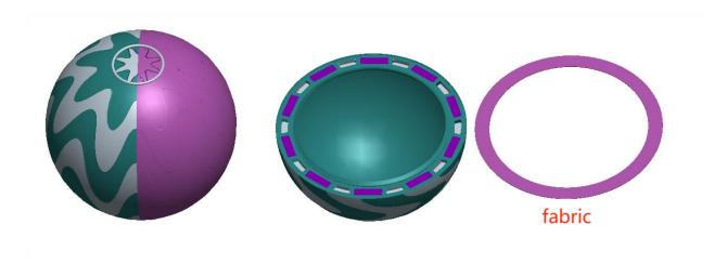
R11 Version (2021.6.23): Changed the outer diameter of the water balloon from 68mm to 58mm.
