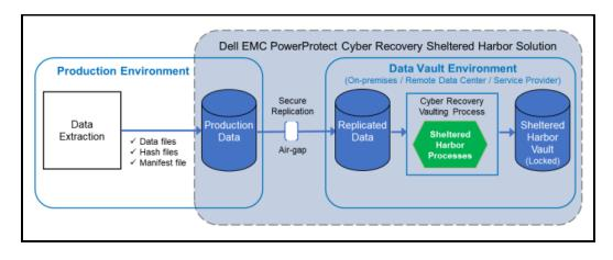
73. The Sheltered Harbor specifications require participants to protect critical data sets, including by creating dedicated, isolated environments which are physically separated from corporate networks and backup systems. Such data sets are converted for storage into Sheltered Harbor standardized format so that basic banking services can be quickly resumed for customers following an attack or failure. *See* Dell Sheltered Harbor Solution Brief.
