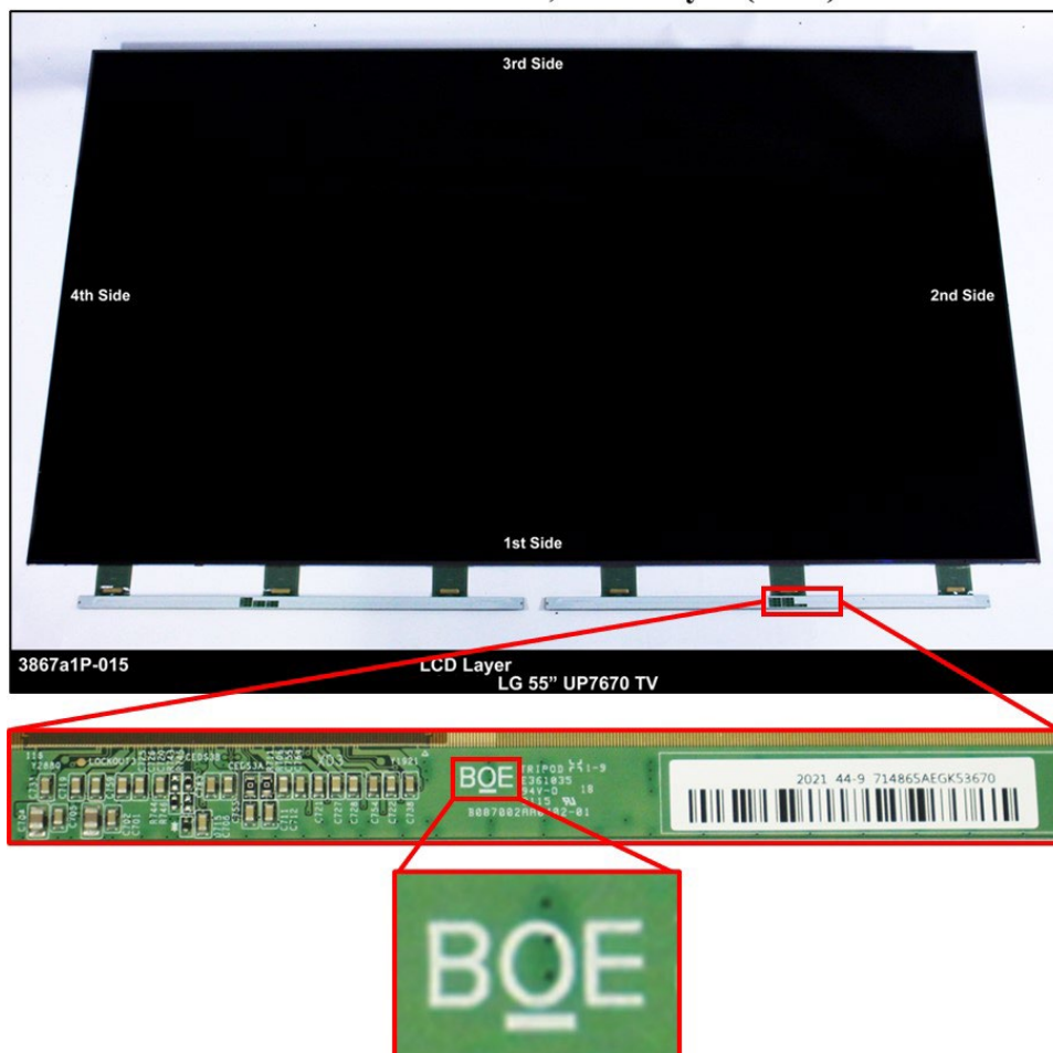
LG 55" UP7670PUC, LCD Layer (front)
