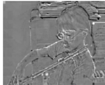
Figure 6.8 Residual after subtracting intra prediction
