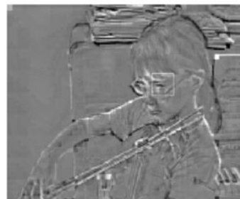
Figure 6.8 Residual after subtracting intra prediction
