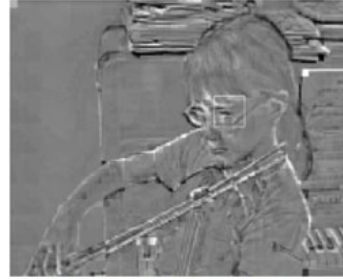
Figure 6.8 Residual after subtracting intra prediction
