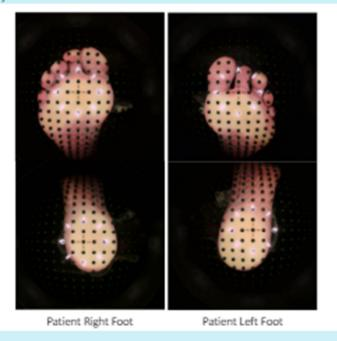
Black dots = patented temperature sensors
