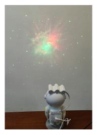
31. To perform lighting effects, the Accused Product includes a light source that projects light through a rotating filter that is powered by a motor. The lighting effects are created by patterns on the filter which do not require the device to manipulate the light source, as depicted in the images below:
