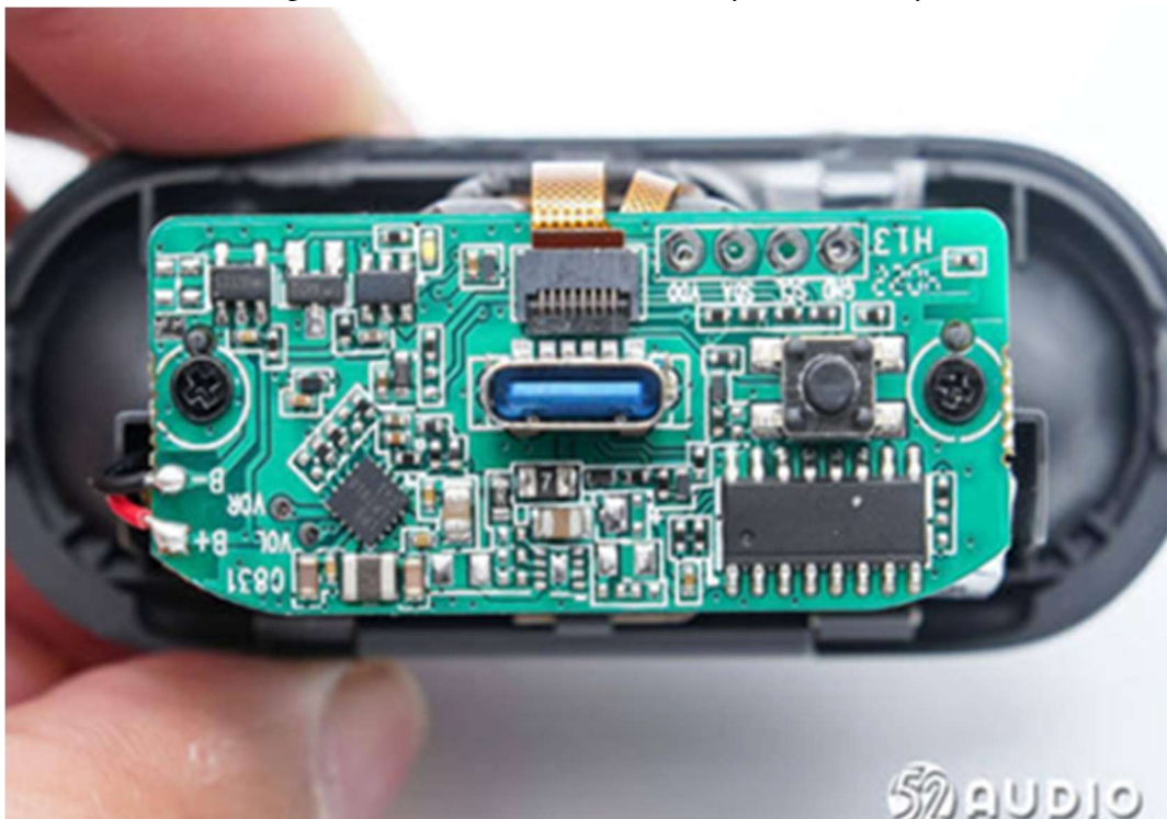
Capsule 3 Pro Base Station Circuitry and Memory
