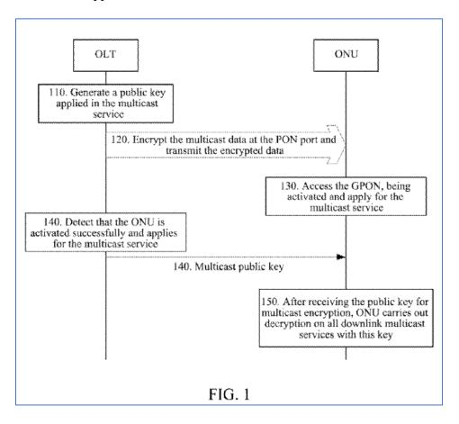
51. The multicast encryption solution provided by '378 Patent provides several benefits for PON networks, including "reduc[ing] the complexities of the OLT encryption mechanism and the ONU decryption mechanism," and "improv[ing] the security of the multicast service content"
