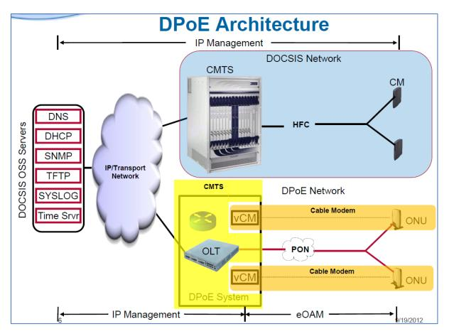
CableLabs, "DOCSIS Provisioning of EPON (DPOE): Architecture, Specifications, Qualifications" at slide 6, available at <a href="https://www.itu.int/dms\_pub/itu-t/oth/06/5B/T065B0000320011PDFE.pdf">https://www.itu.int/dms\_pub/itu-t/oth/06/5B/T065B0000320011PDFE.pdf</a>.
