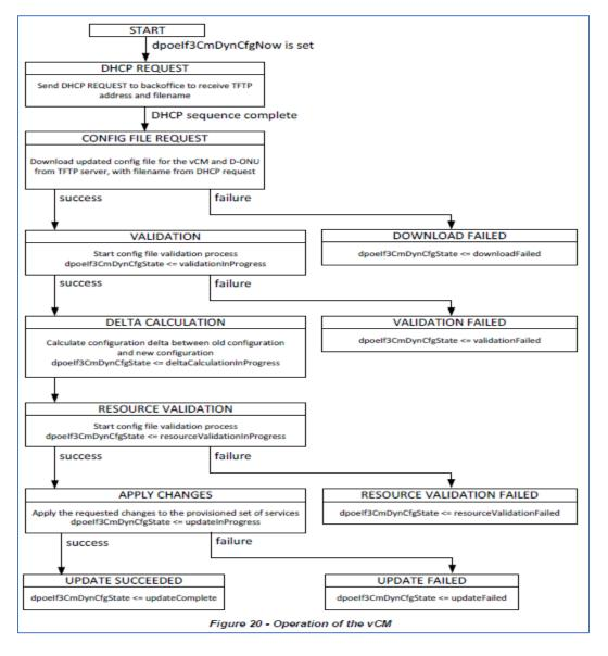
80. The Accused Instrumentalities include the claimed "receiving a notification that an updated configuration file is available for the ONU, wherein the ONU is configured with a current configuration file." For example, the DPoE v2.0 specification explains that the DPoE System
